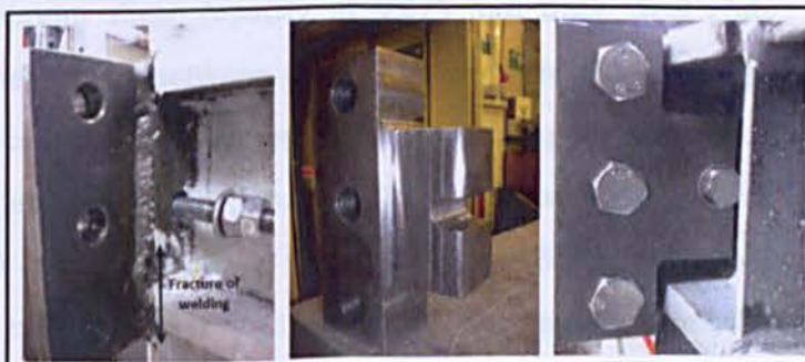
Figure 4.35: Utilising rigid clamp plates prevent damage of welding at location of connection between loading plate and column's outer flange
