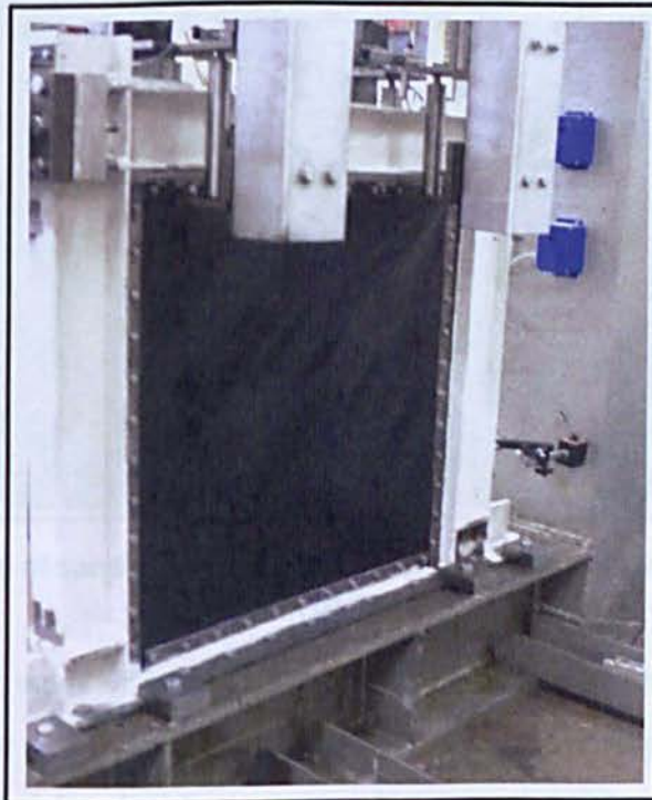
Figure 5.34: Initiation of elastic buckling noted during cycle #13 for W1G1 specimen
