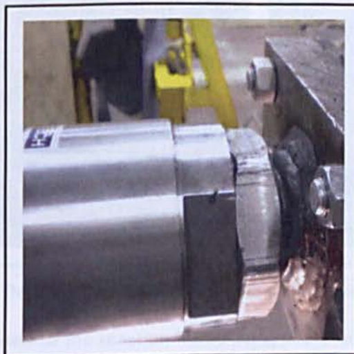
Figure 4.29: Tightening the lock nuts when system is running under tensile loading
