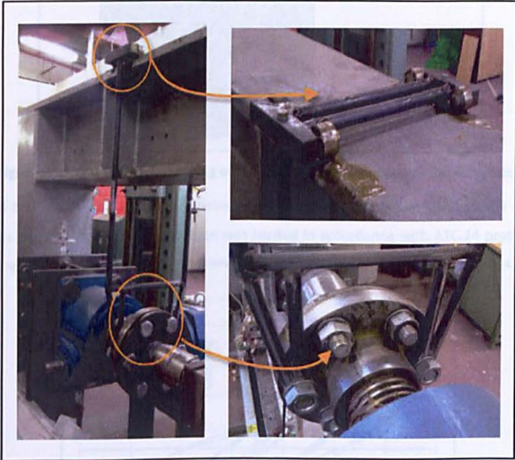
Figure 4.36: Anti rotation hanger prevents any rotation to be applied to the test specimens
