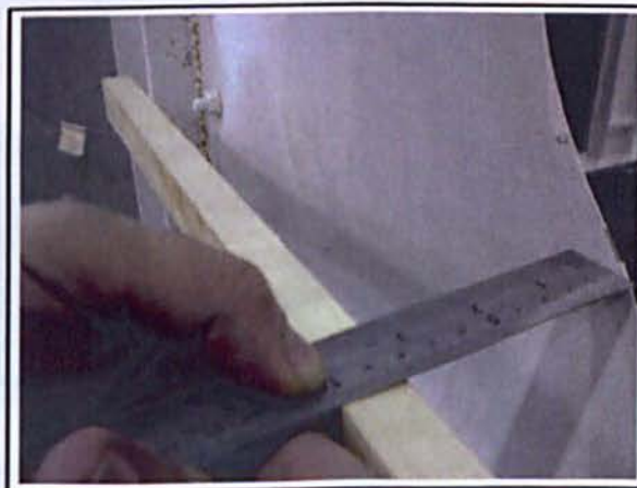
Figure 4.26: Manually measurement of out-of-plane buckling of steel plate
