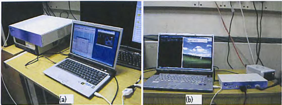
Figure 6.3 WiMAX experimental testbed. (a) Mobile WiMAX base station and ultrasound video streaming node; (b) CPE and ultrasound video receiver node
