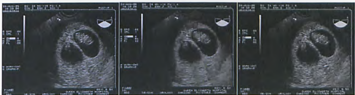
Figure 6.7 Ultrasound images PSNR 38.86. (a) Original image. (b) Received image over HSUPA network. (c) Received image over Mobile WiMAX network
