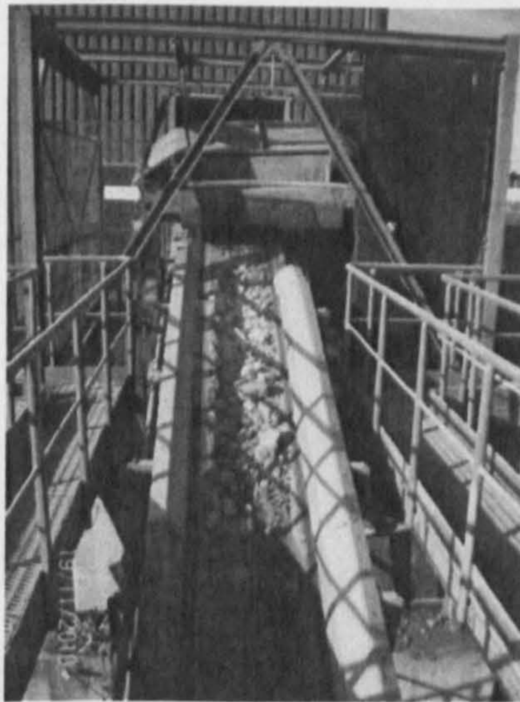
Figure 4.17 A belt conveyor in Day Group plant conveys the aggregate into screens (photograph courtesy of Day Group Ltd)
