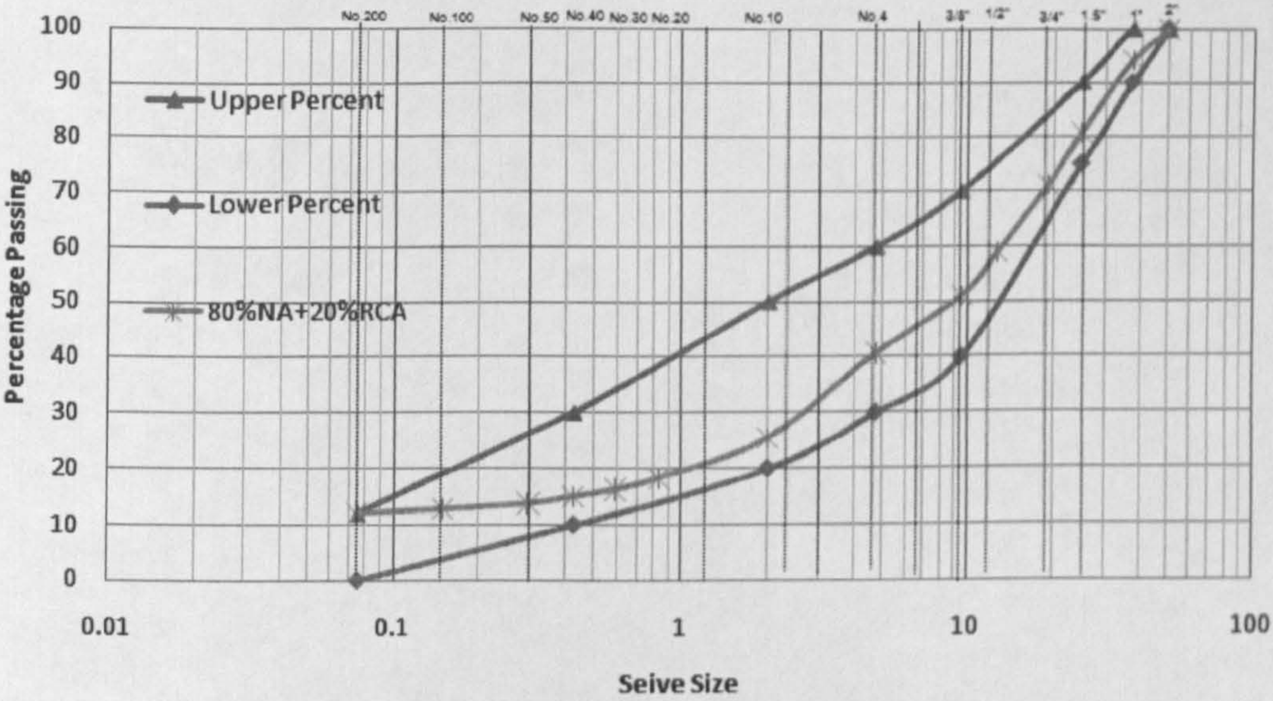
Figure 5.44 Grading curve of 80%NA+20%RCA
