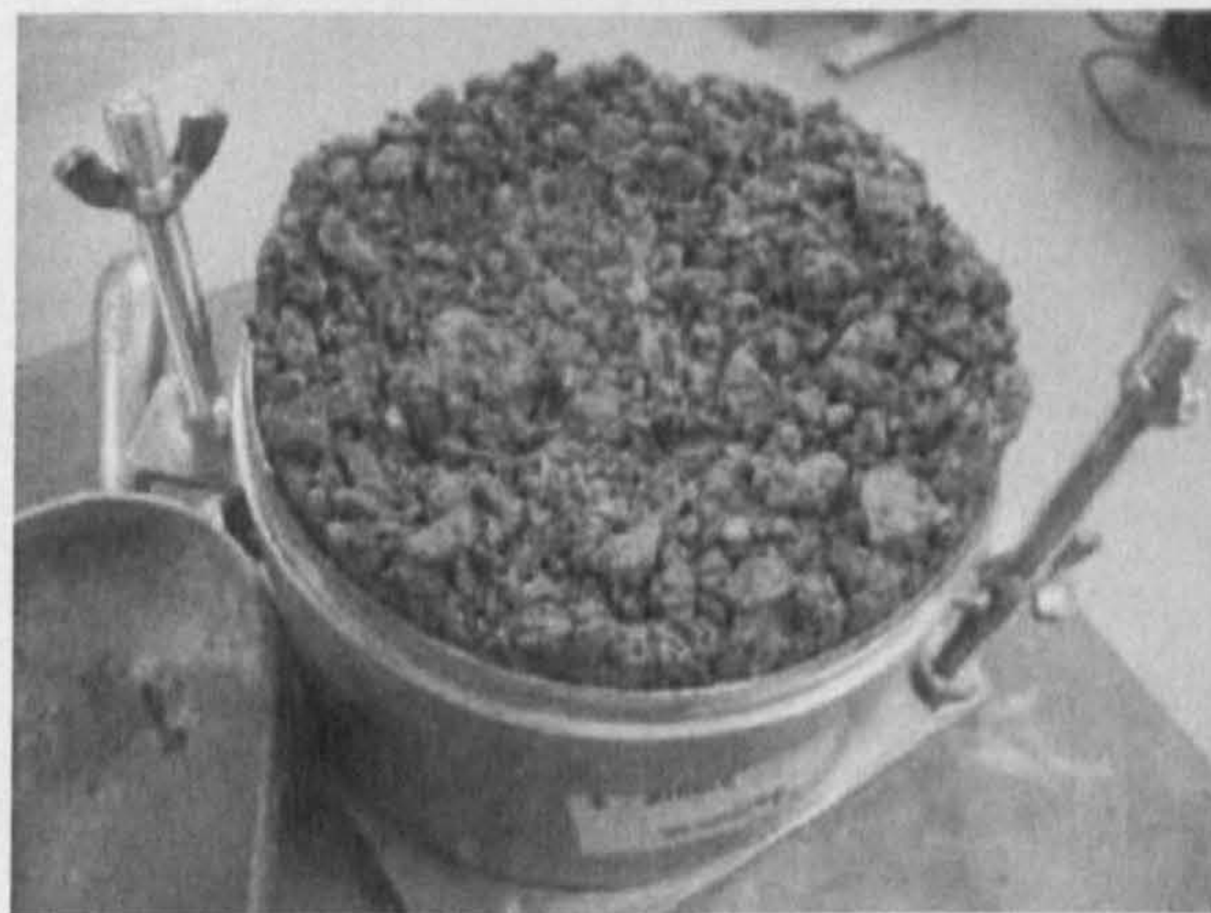
Figure 5.29 Apparent segregation irregularities in T-2 (100% NA) before CBR test
