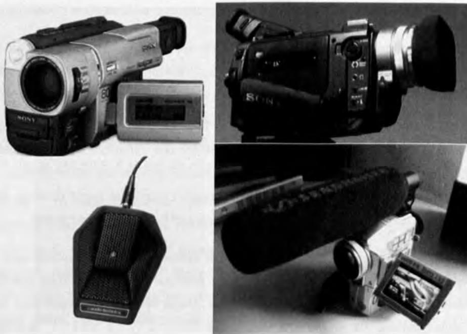
Figure 3.5: Video recording hardware; Analog (top left) and digital (top right) cameras using tapes as storage medium, a multidirectional desktop microphone (bottom left) and a mono-directional microphone mounted on a camera
