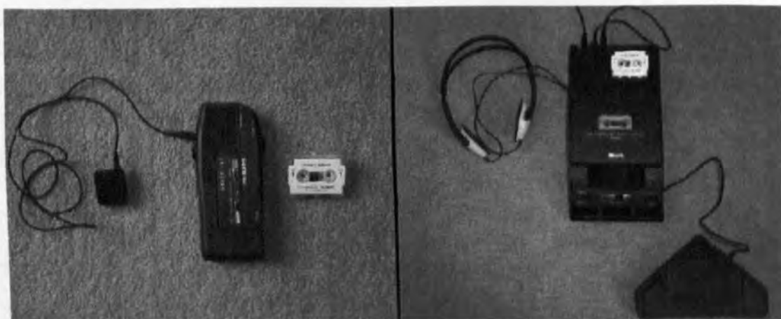
Figure 3.3: Dictaphone with external microphone (left) and transcription machine with foot paddle controller (right)
