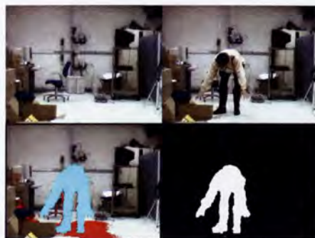
Figure 2.1 – Example of shadow detection and removal (taken from [45]). Upper left: background model; upper right: input frame; lower left: output from background subtraction (foreground is blue, shadows are red, highlights are green and background pixel are kept in the original colour); lower right: foreground region after shadow removal is performed.
