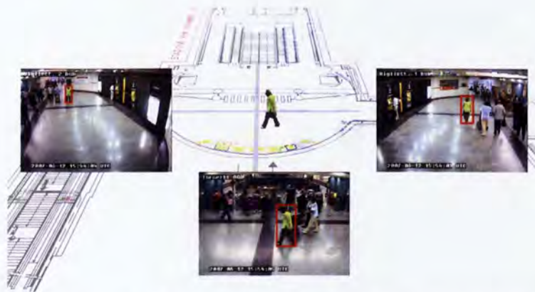
Figure 3.1 – Targets and individuals. The map of the underground station in the background represents the real world, where several individuals are present (to avoid cluttering the image, only one individual \hat{i} is shown, wearing a yellow top). The real world is imaged by three cameras (inset left, centre and right). In each camera, there is a target i_{1,2,3} (highlighted with a red bounding box) corresponding to this individual, plus other targets corresponding to other individuals. Because all targets i_n correspond to the same individual, we can write i_1 \equiv i_2 \equiv i_3 .
