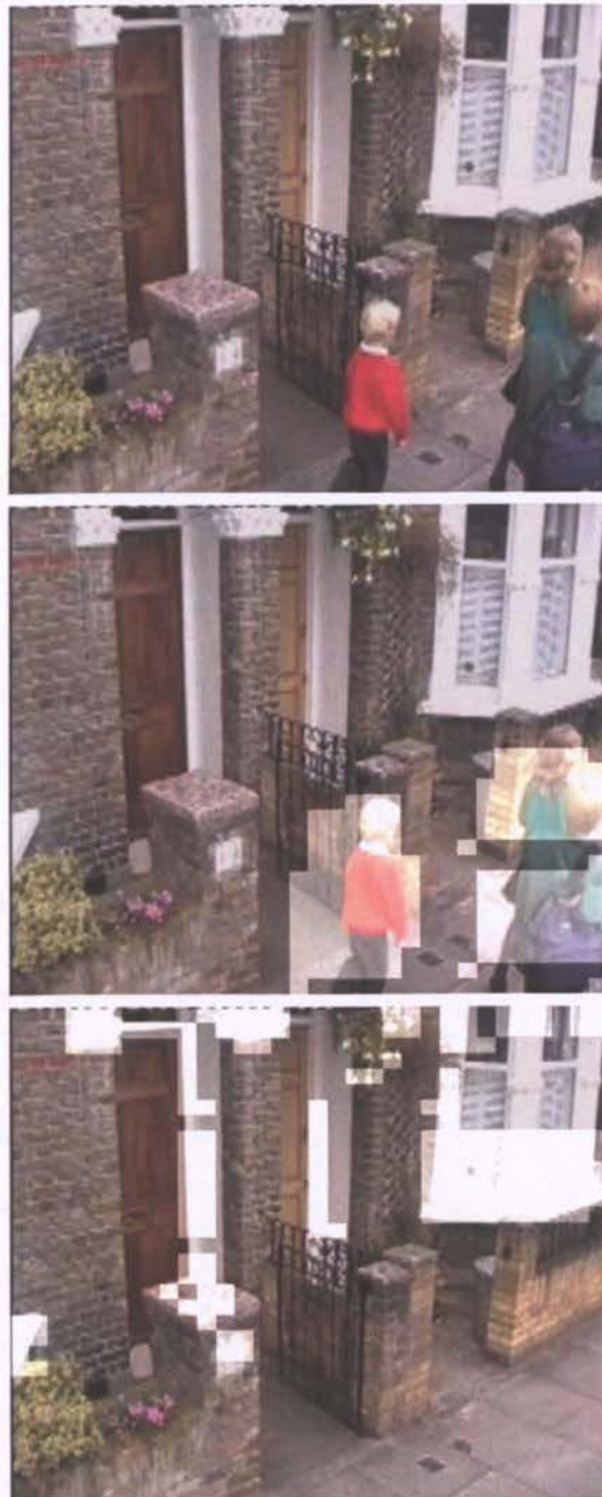
Figure 6.5: The Overview data set showing moving people (top), corresponding motion masks (middle) and an example of errors in the motion detection (bottom).
