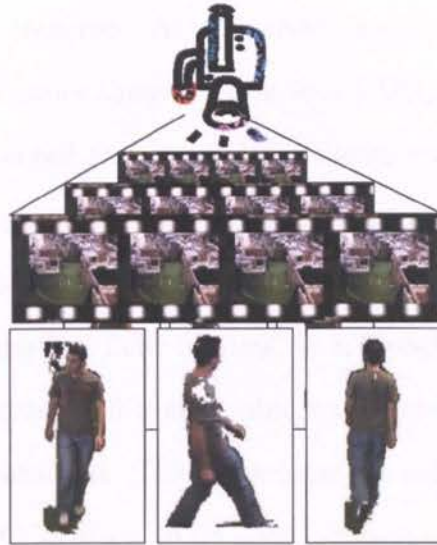
Figure 5.4: The camera sensor produces meta-data about the Low Level Objects (LLOs).
