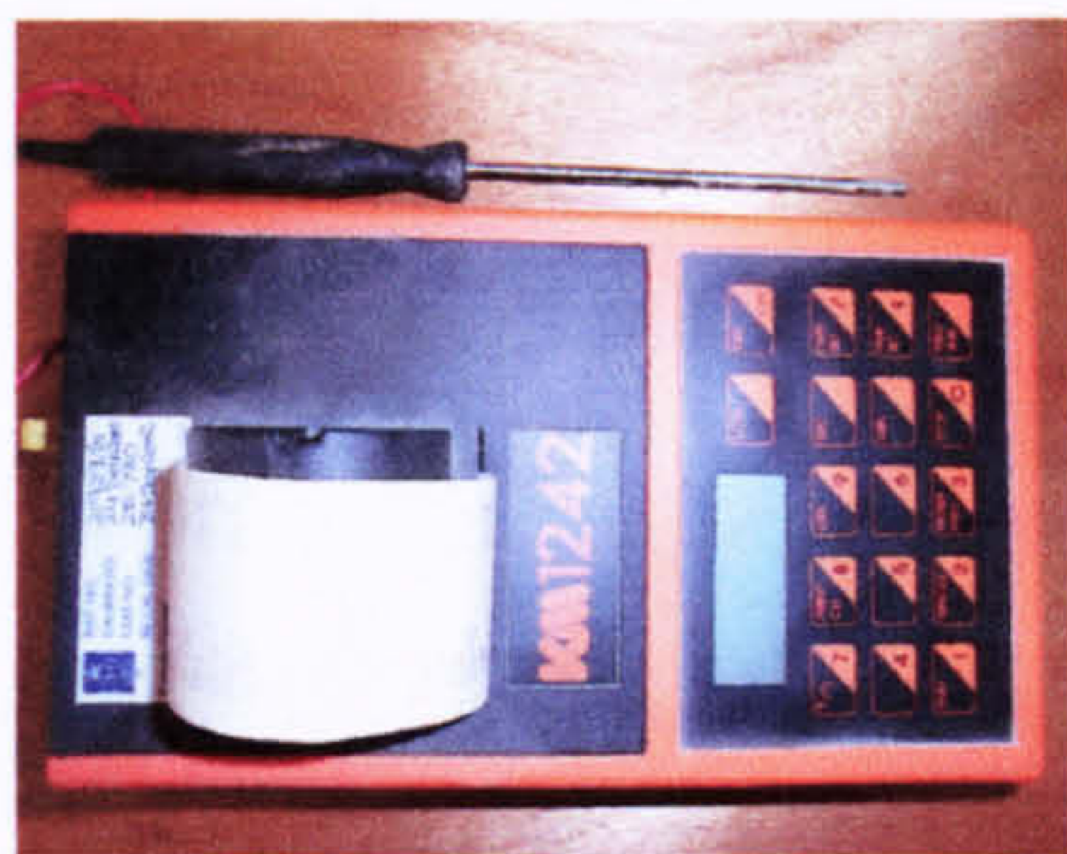
Figures 11.3 the data loggers used for the heat of hydration work
