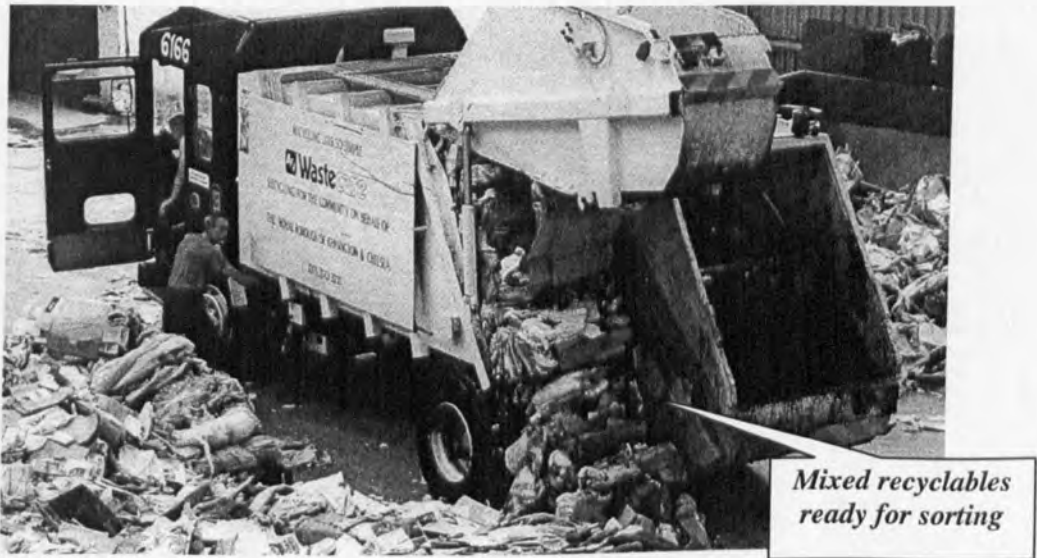
Figure 5.7. Split back vehicle tipping at the MRF (source: author)
