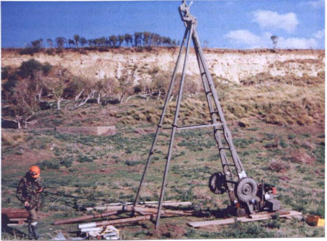
Plate 6.5. The pilcon cable percussion rig.
