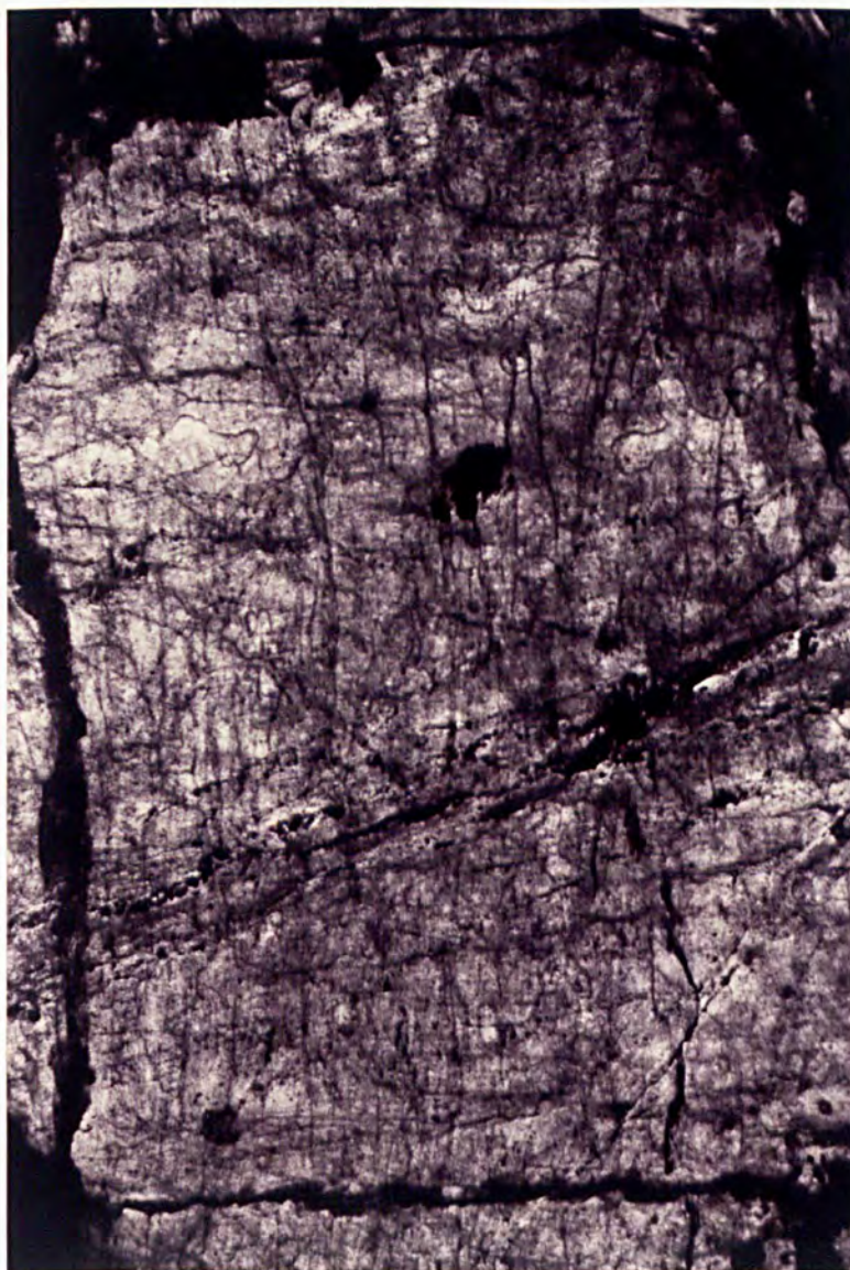
Plate 4.1 Quartz crystal from Lee Moor kaolinised granite (approx. 5% kaolinite alteration) exhibiting high FIP abundance. Note the presence of intracrystalline FIPs forming two sets at 90^\circ and the large intercrystalline shear fracture in the bottom right hand corner.
