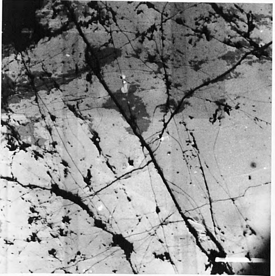
Plate 5.9. SEM-CL image of a alkali feldspar from sample WBN1 (Dartmoor granite). Various generations of FIPs are easily identifiable based upon varying intensity and grey scale contrasts. Width of frame is 2mm, vertical edge aligned 000^{\circ} (due north). Section cut in the horizontal plane. Note the large intergranular fracture (bottom right to top left) exhibiting dextral shear (off-setting of earlier) and possible strike-slip duplexes.
