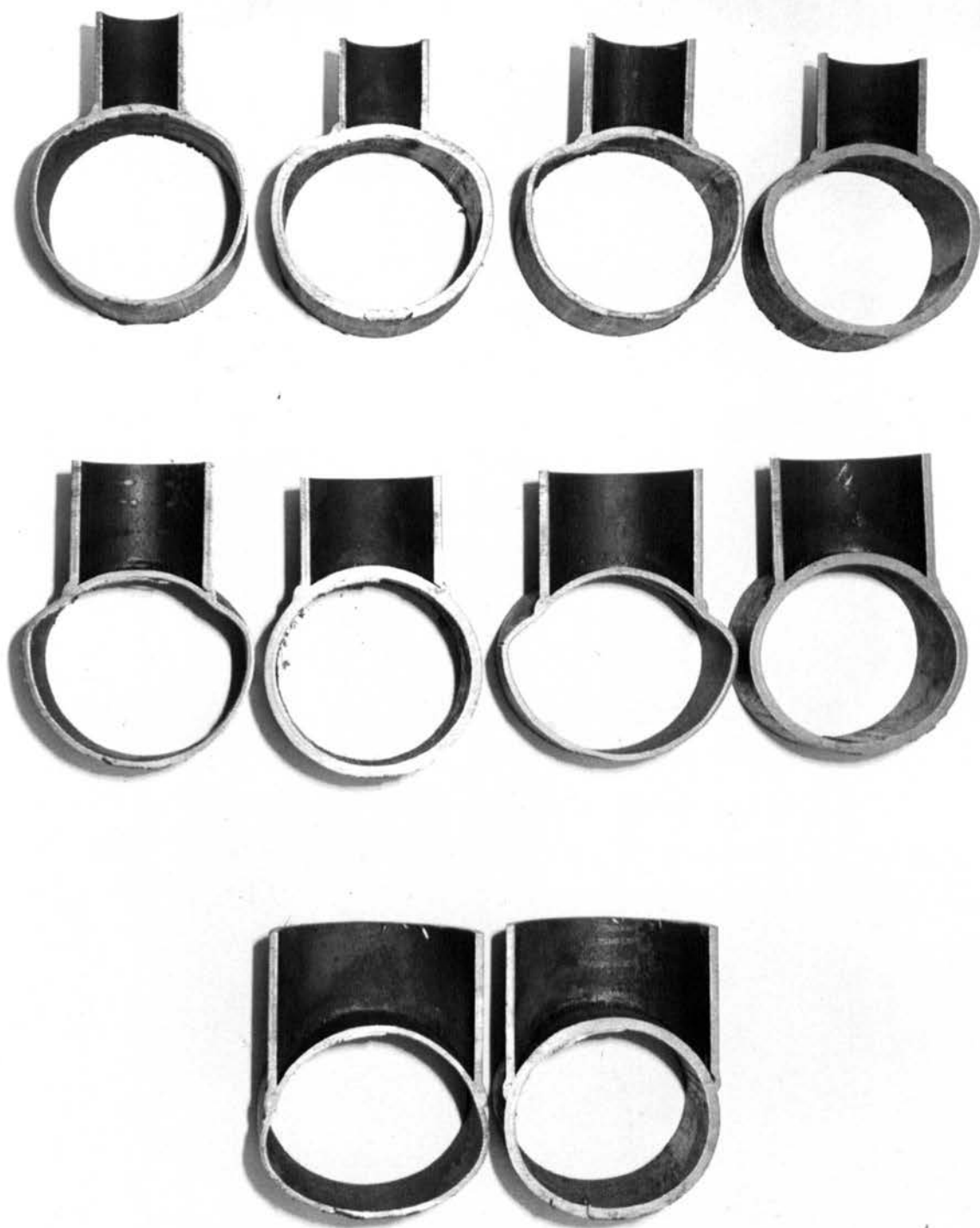
Figure 172 - T-Joints Subject to Axial Load ( \beta = 0.42 - 1.0 ) d_o/t_o = 32 , d_o/t_o = 18
