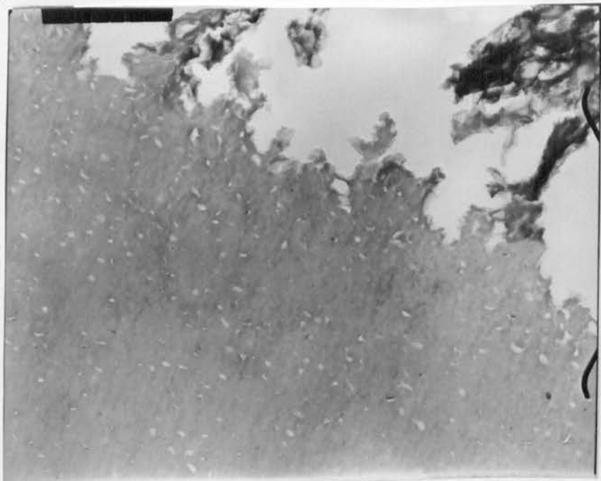
PLATE 15 Sample of Resin 5 Exposed to Water for 10 Days 19K, x 51,000
