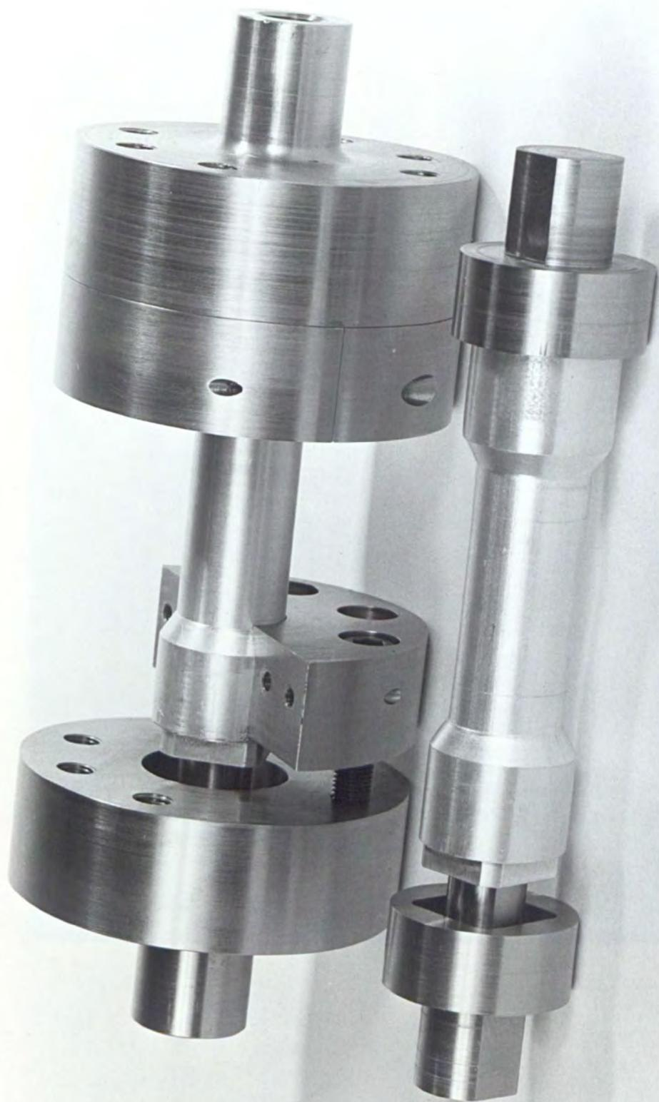
Fig.2.16B Tension & Torsion Prestrain Adaptors
