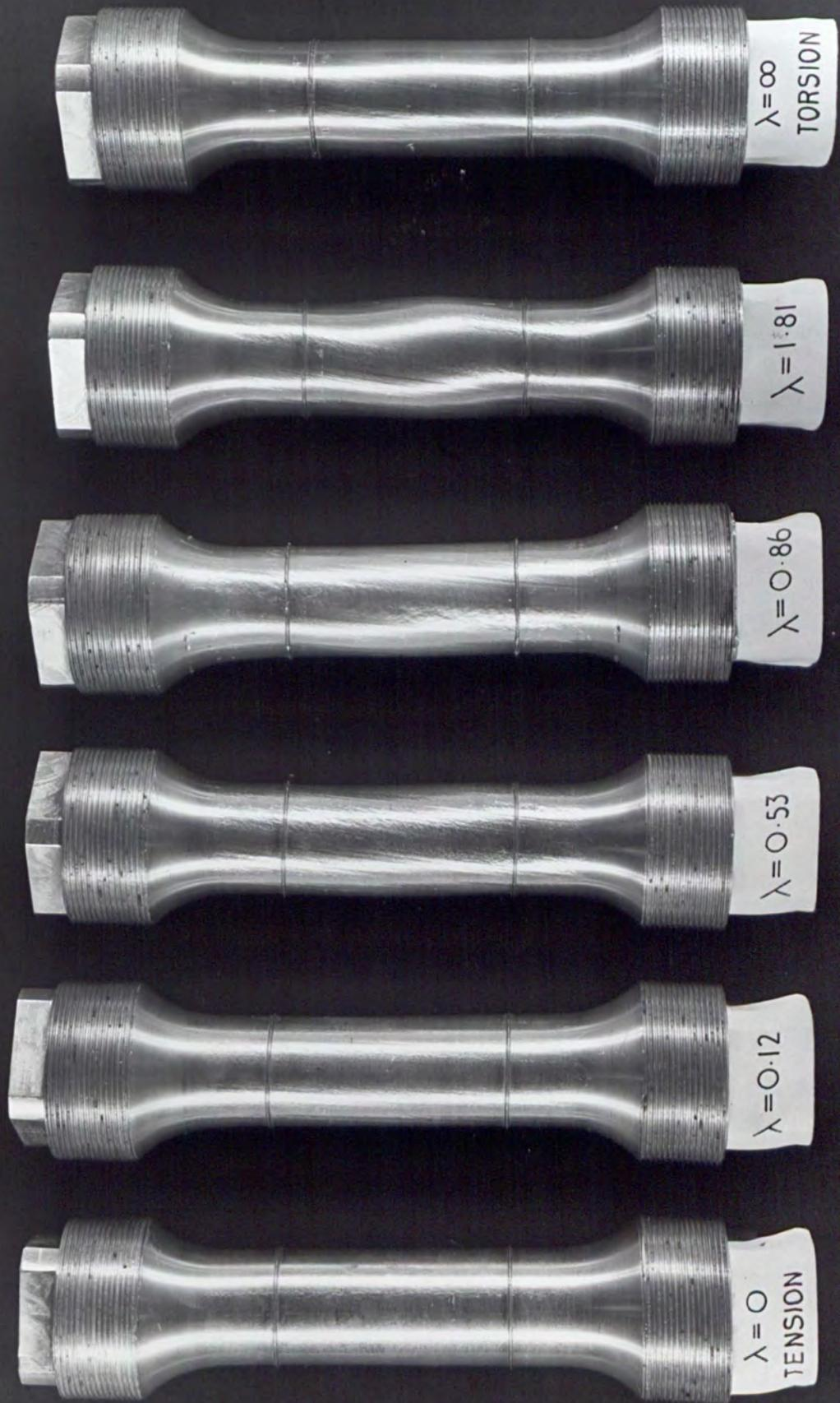
Fig. 4.13 Constant  $\lambda$  tubular specimens
