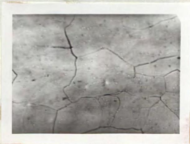
Fig.13 Grain boundary sliding
