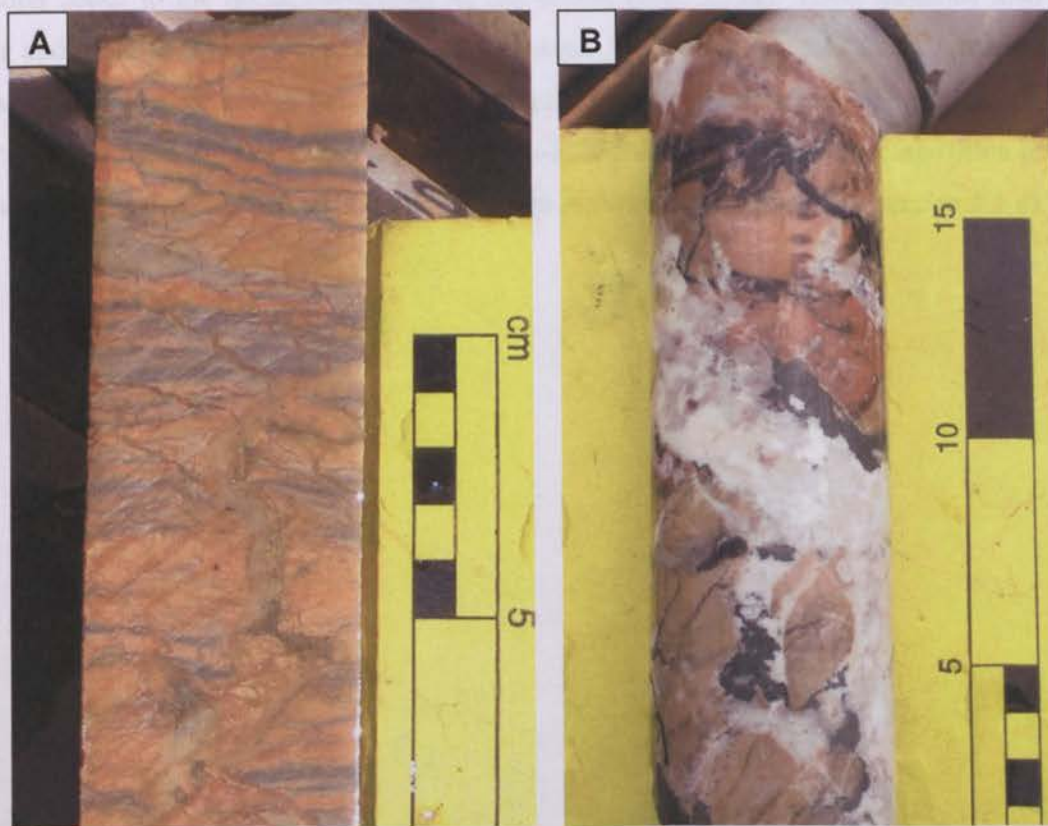
Fig. 5.12. Drill core photos of phyllic alteration at Yalea Main. A) Green sericite-chlorite shears overprinting pink albite altered rock in proximity to the orezone (YDH132, 534 m). B) Chlorite-carbonate-quartz veins cross cutting albite-altered rock. (YDH187, 350 m).
