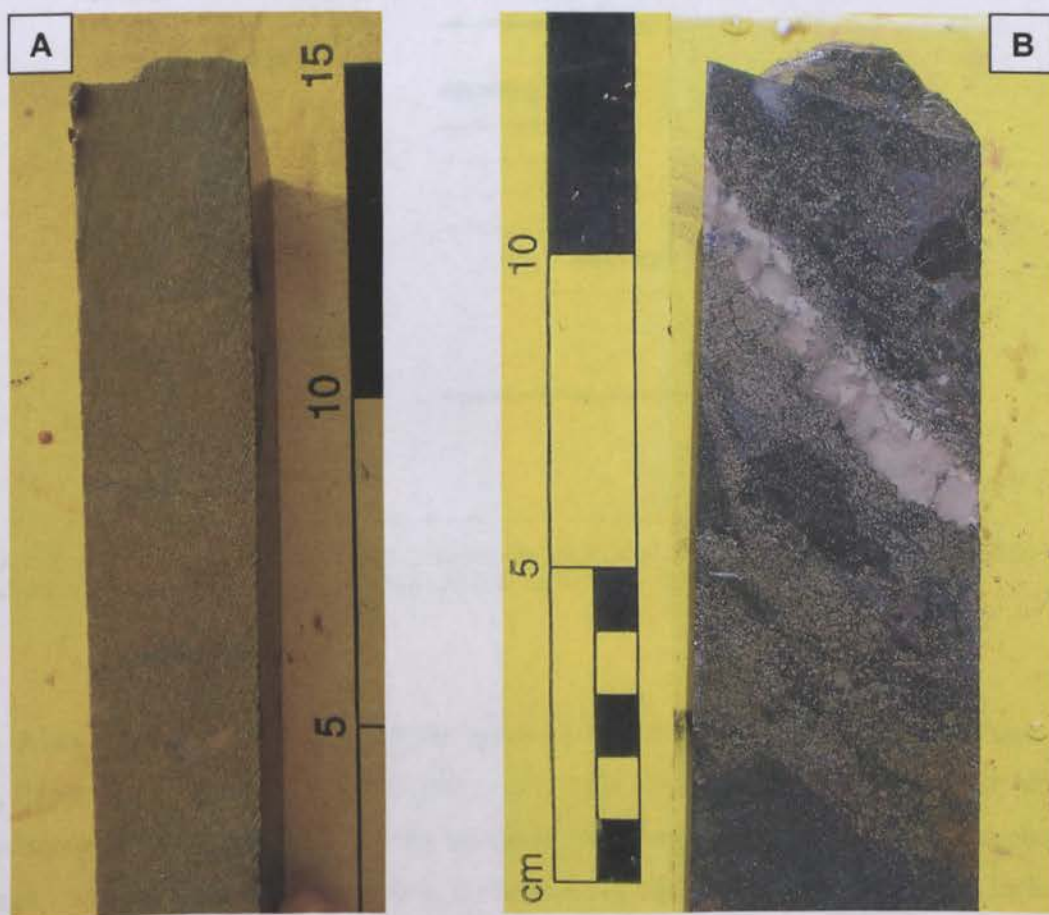
Fig. 4.14. Drill core images showing the main mineralisation style at P-125. A) Massive disseminated sulphides (pyrite and arsenopyrite; the latter too fine-grained to see with the naked eye) (P125DH12, 141 m). B) A weaker disseminated zone showing clearly the presence of both pyrite (70%) and arsenopyrite (greyish minerals; 30%). Arsenopyrite contains a brown halo where they have altered to goethite. Disseminated sulphides cut across a weakly mineralised quartz-carbonate vein (P125DH12, 154.9 m).
