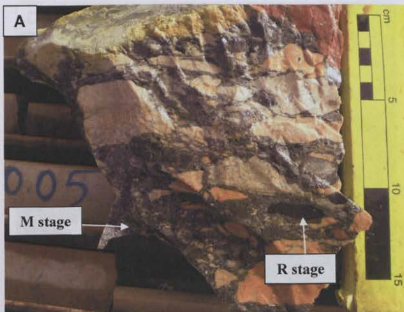
Fig. 5.6 A). Hydrothermal-tectonic breccia host rocks at Yalea North (modified from Fig. 3.11; rock descriptions in section 3.3.5 ). Tourmaline occurs within the matrix of the breccias along with mineralisation (M stage) or as reworked material (clast fragments between 200 \mu\text{m} to 5 cm; R-stage). Multiphase tourmaline growth is clearly distinguished in the photomicrographs shown below.
