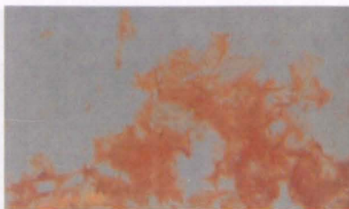
Figure 24. The golden brown precipitate of a 1:1 Cu(II) ions and 6G solution.
