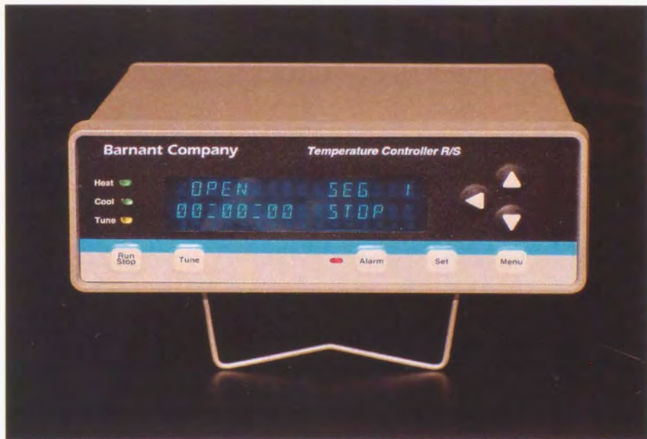
Figure 3-5a Temperature Controller for tube furnace
