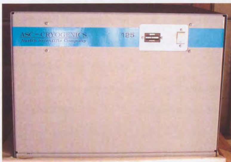
Figure 3-6 Cryogenics refrigerator compressor
