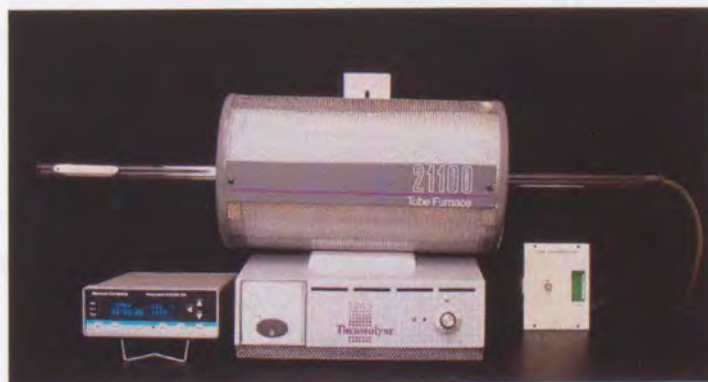
Figure 3-3 Thermolyne Tube Furnace with ceramic boat inserted at left end of tube.
