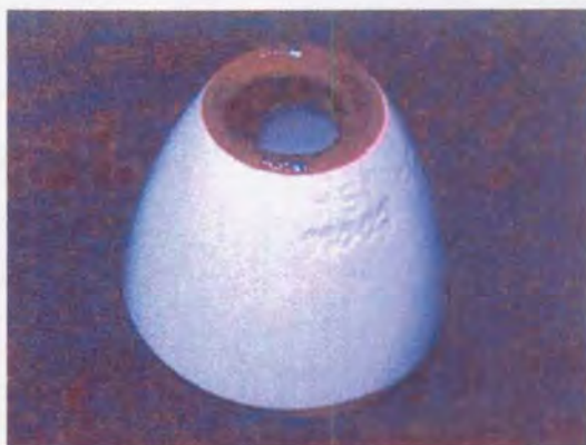
Figure 5-5 Hole in bottom of crucible which through sample pellet melted.
