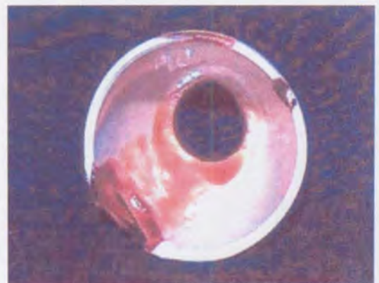
Figure 5-6 Inside of crucible showing melted path where sample pellet slid down inside.
