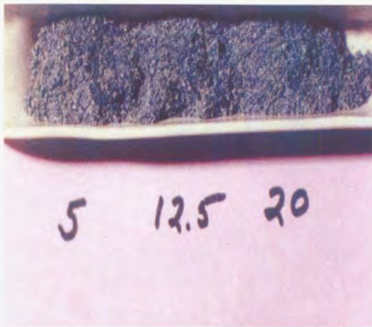
Figure 5-3 Same disintegrated pellets showing that 2.2, 5.7 and 89.1 kN pelletizing force made no difference in structural integrity.
