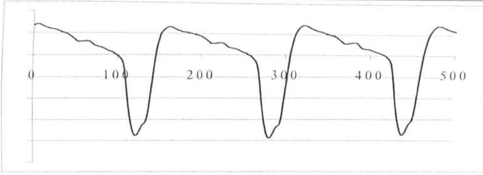
Figure 5.8 Signal 1, unrestrained shaft rotating at 65 Hz.
