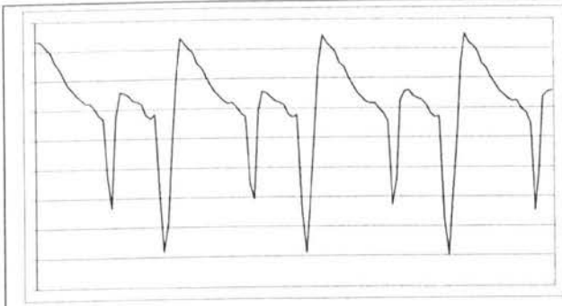
Figure 4.42 120 out of 1024 points of signal resulting in spectrum with many harmonics.
