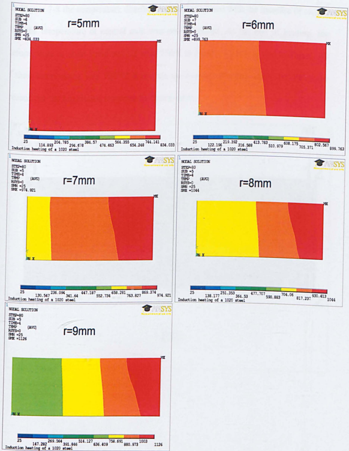
Figure 7-8 Temperature distribution at the end of heating for samples heated at different air-gaps (=10- the radius of sample) in radial direction
