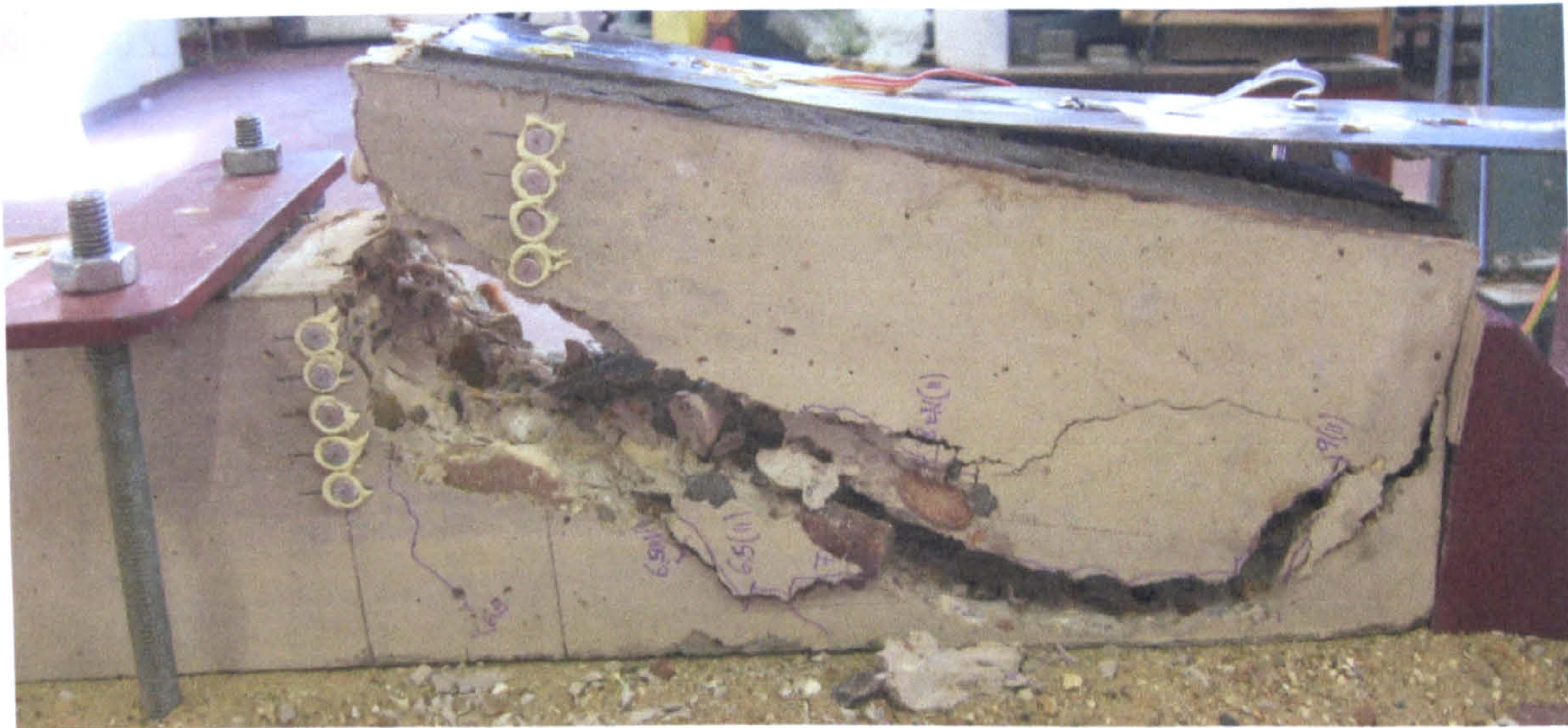
Figure VI-14 Deformability of a sample, group 250°C
