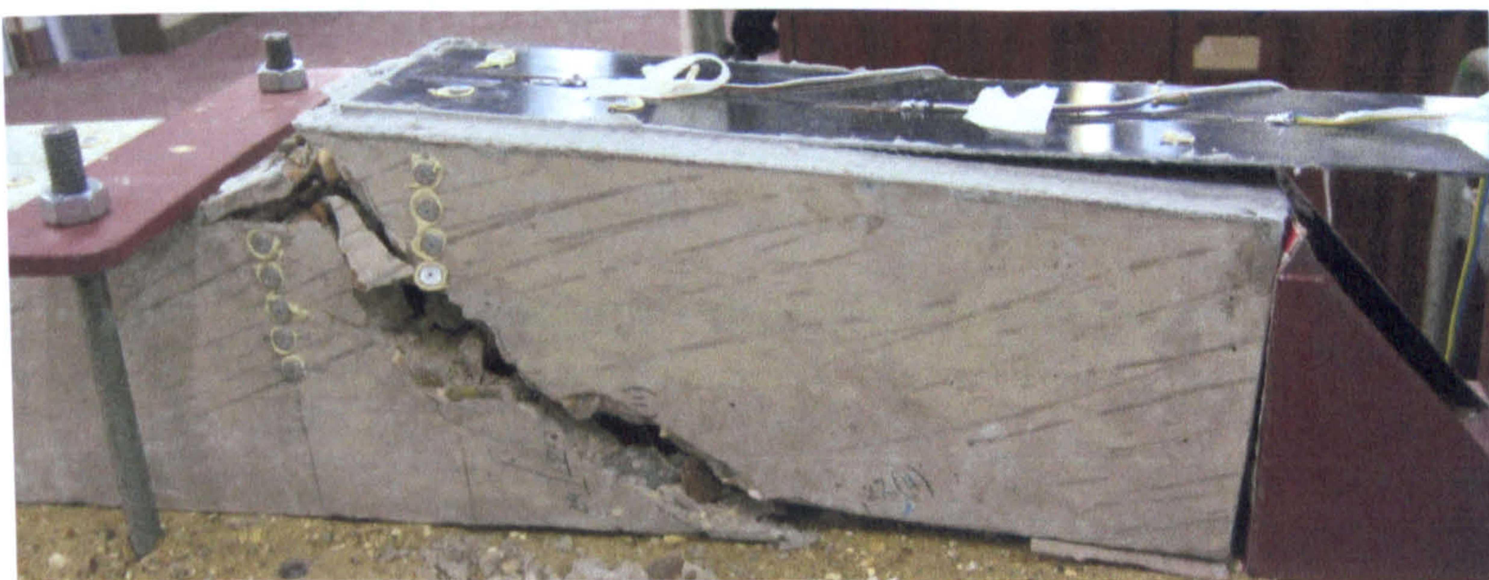
Figure VI- 15 Deformability of a sample, group 50°C
