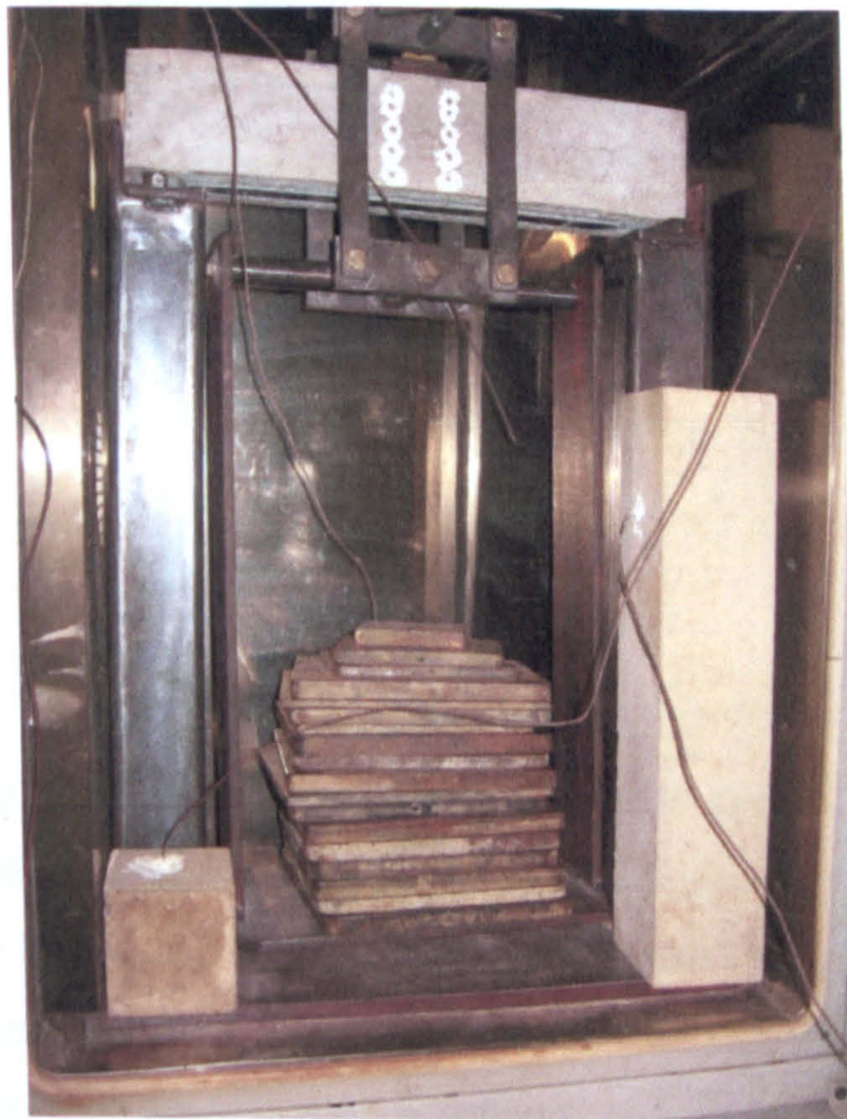
Figure IV-2 Position of the thermocouples and applied load
