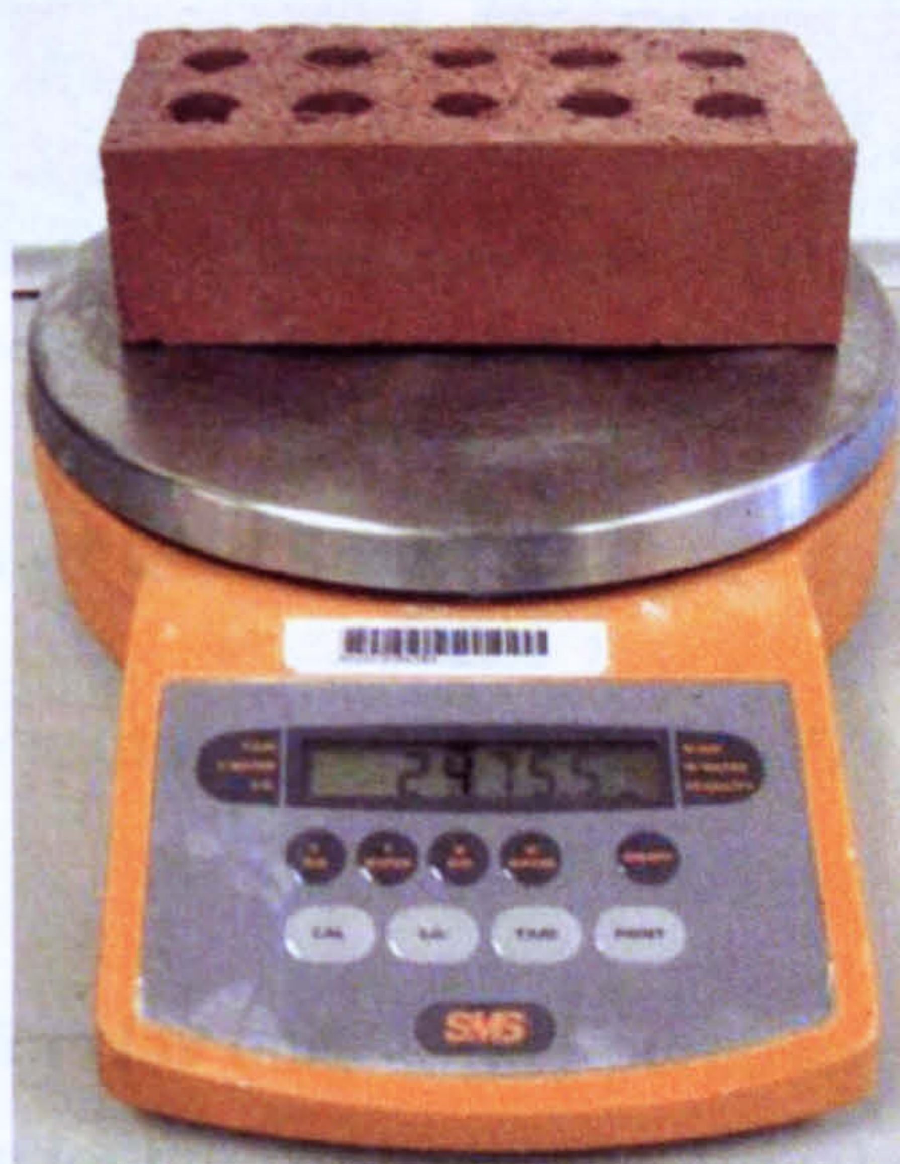
Figure 4.3.1.2 – IRA test – Brick being weighed
