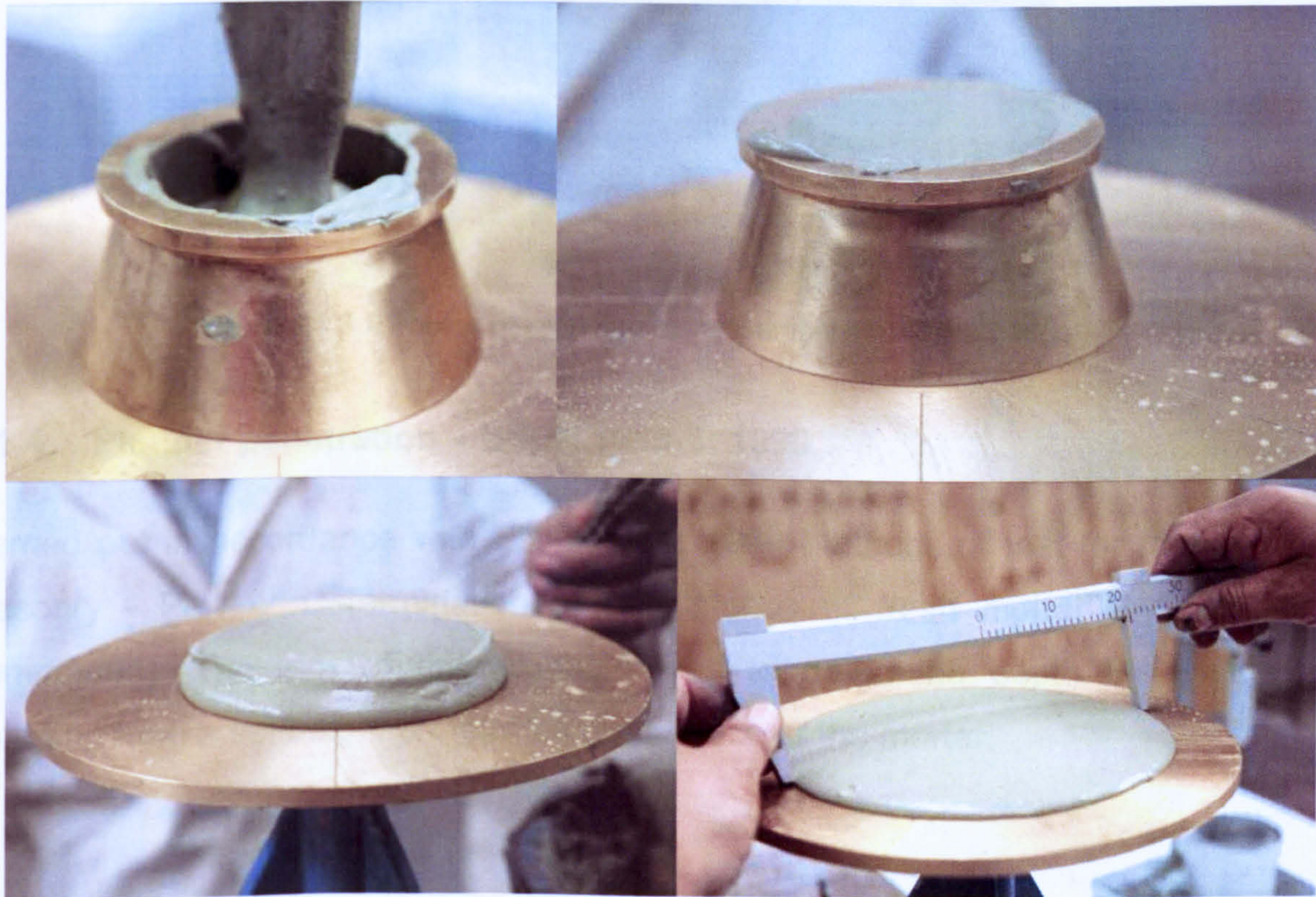
Figure 4.1.2.3 – Photos of preparation and measurements of flow table test (BSEN1015-3)
