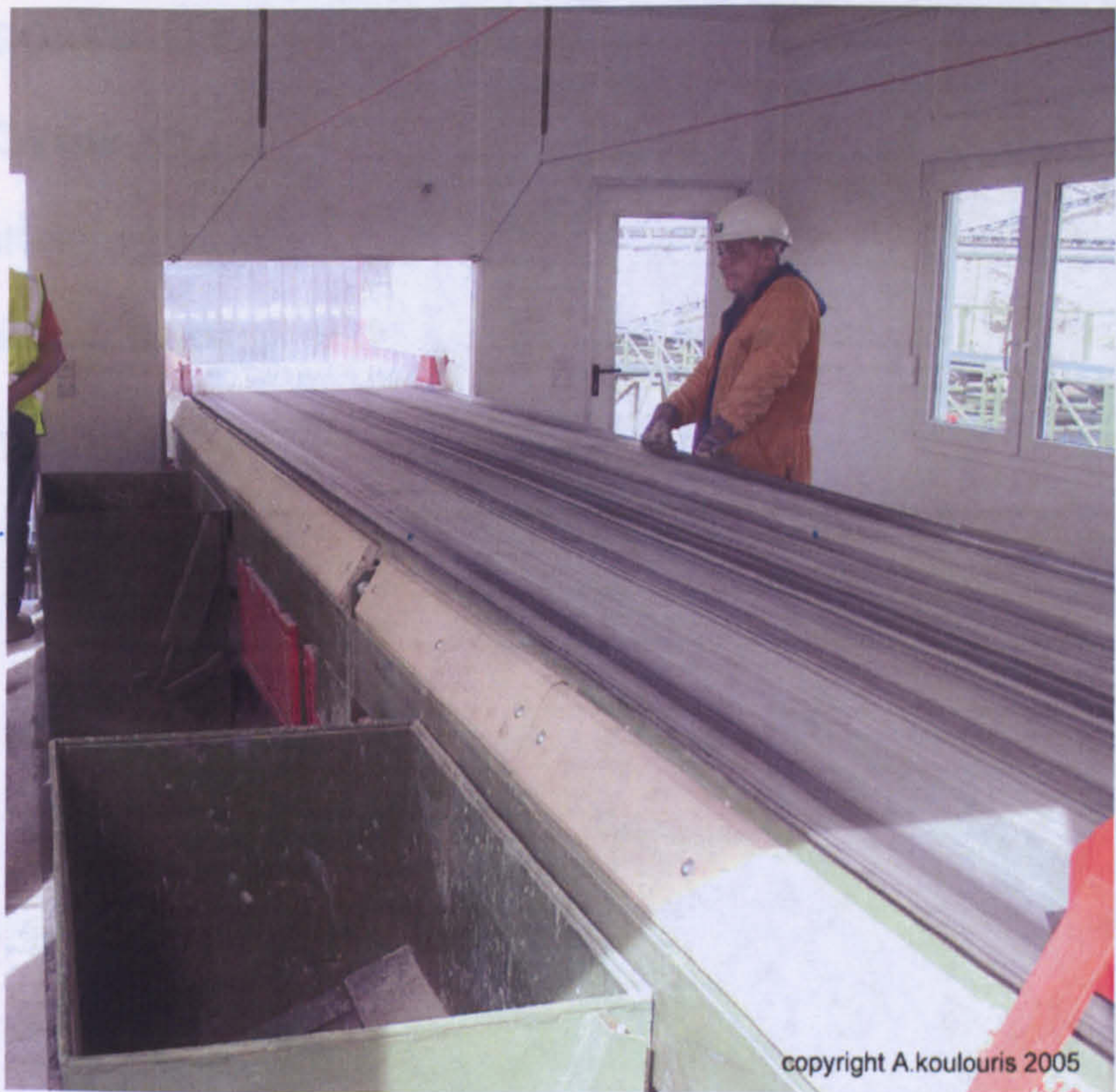
Figure 4.5 Sorting room used for manual removal of foreign materials.
