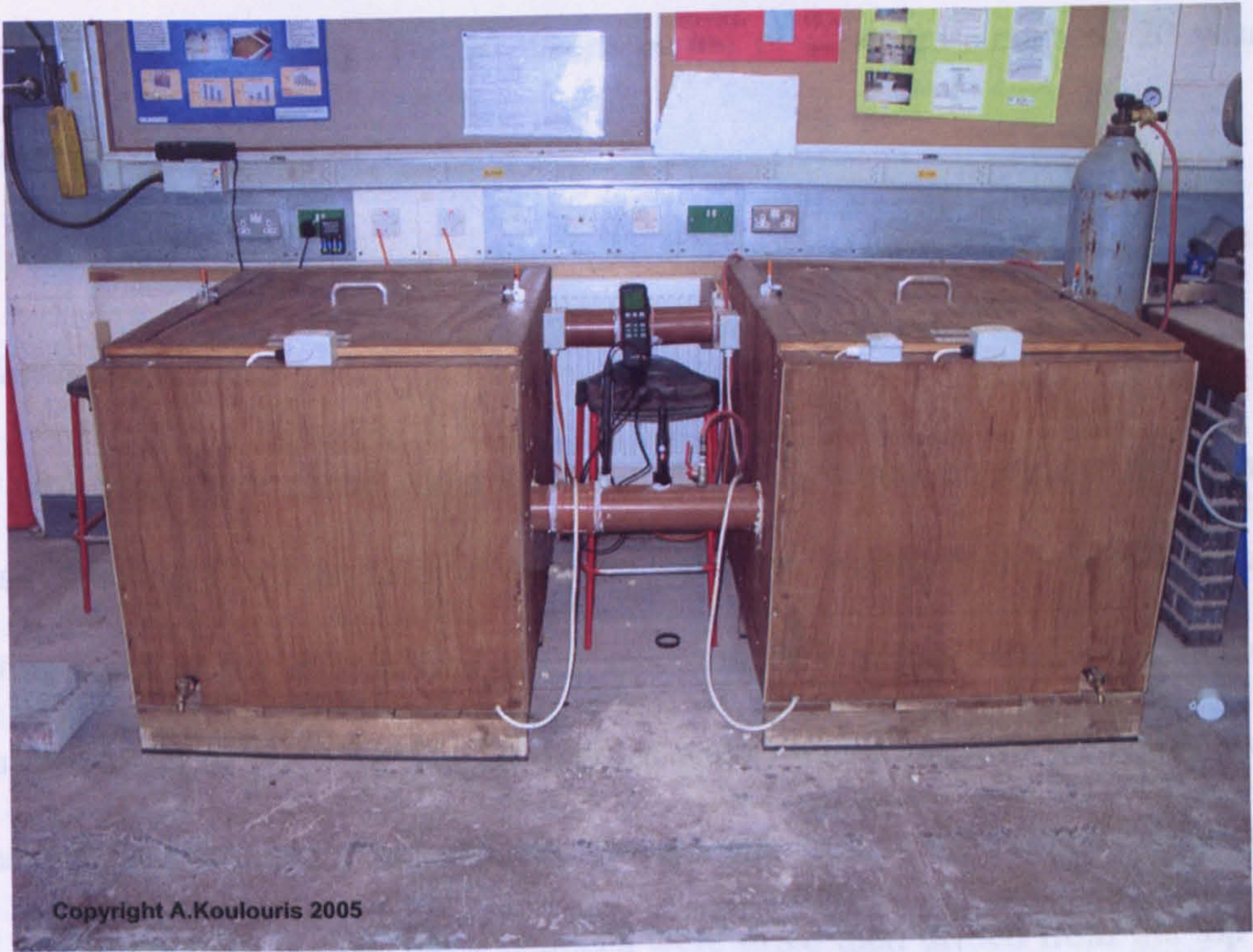
Figure 3.7 Apparatus for carbonation resistance testing.
