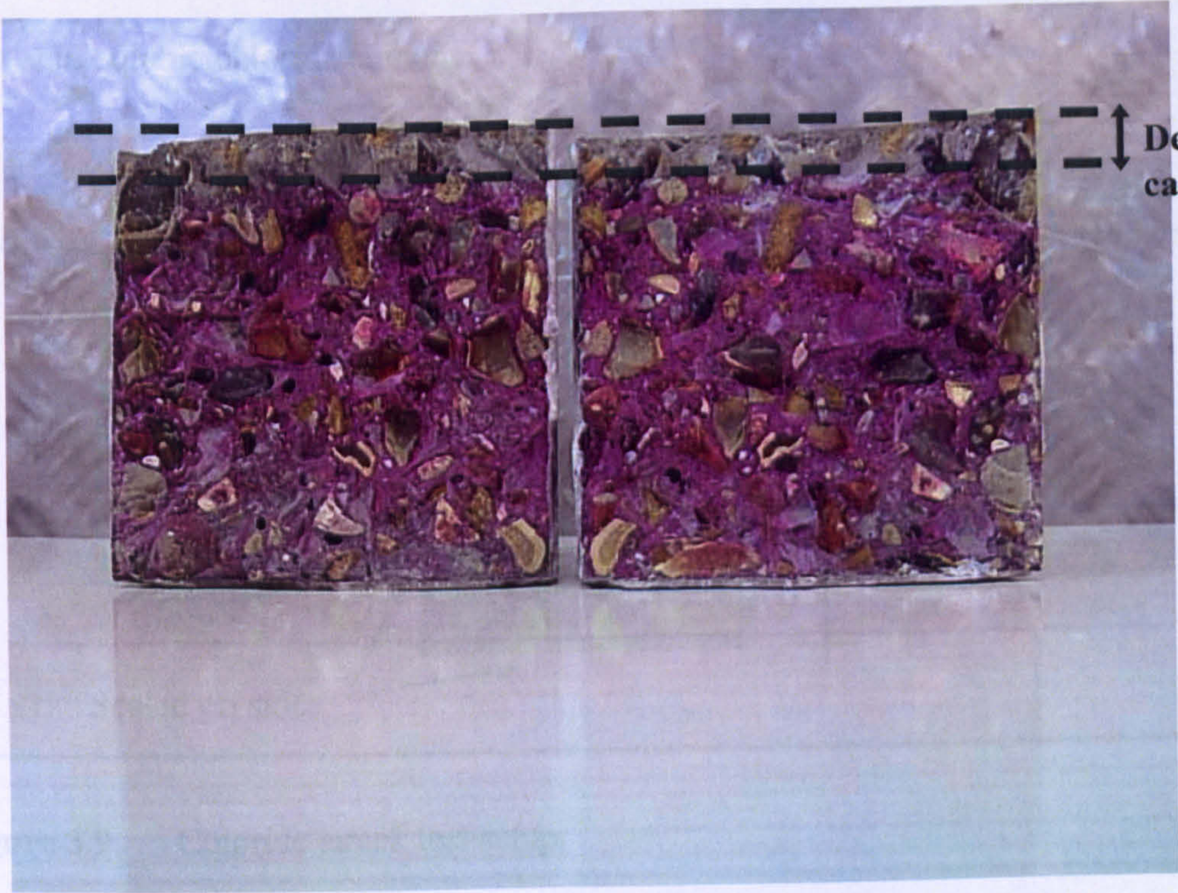
Figure 3.8 Concrete cubes after being sprayed by phenolphthalein solution to reveal the depth of carbonation.
