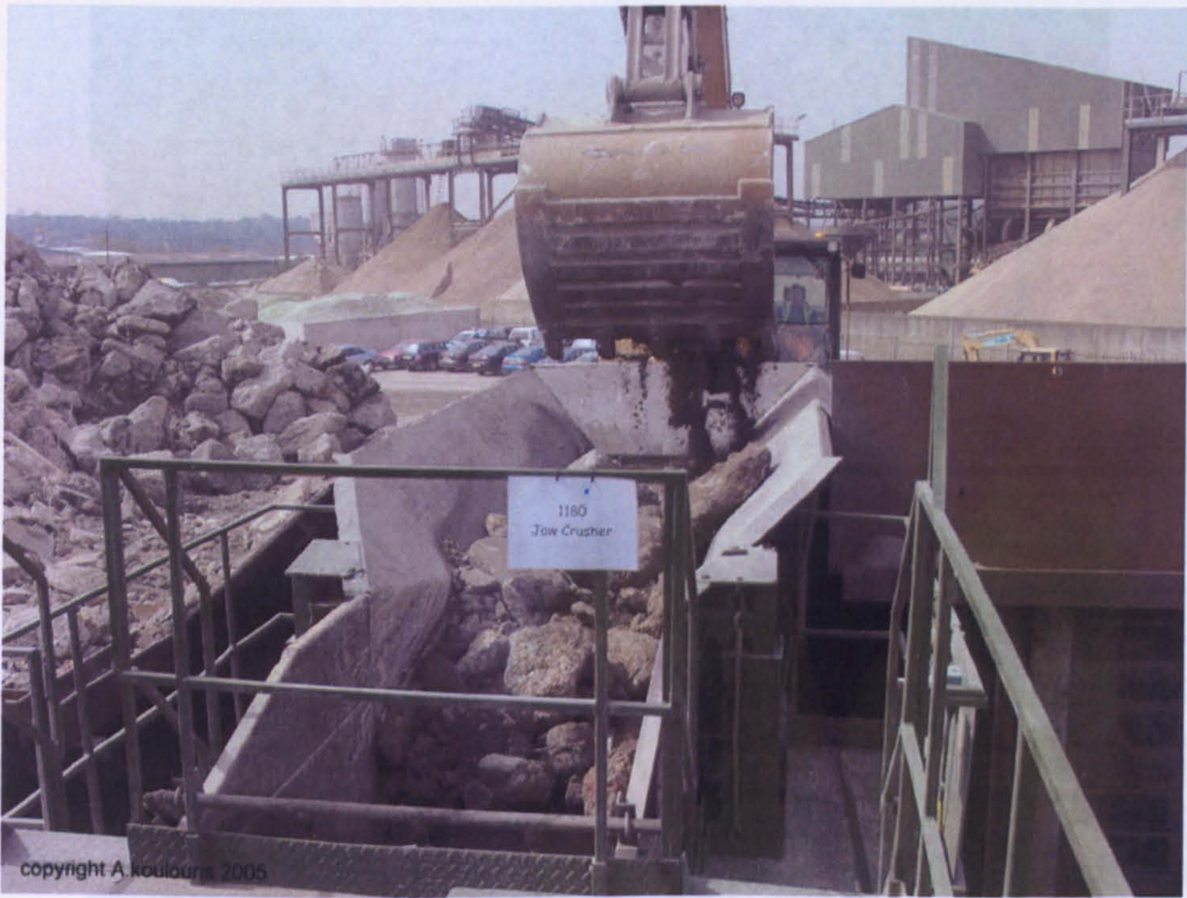
Figure 4.3 Primary jaw crusher reducing C&D debris from 0.4 m to 75 mm.
