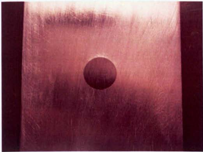
Figure 2.3.2 Specimen with an interference fit fastener
