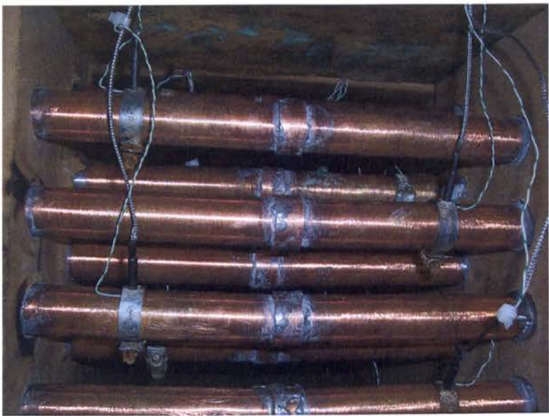
Fig (4.14a) Measurement of the Evaporator Tube’s Surface Temperature
