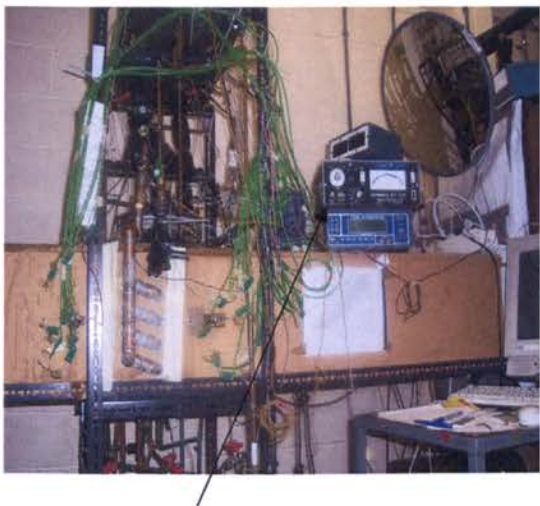
(b) The two pitot tubes are connected to this manometer for measuring air velocity
