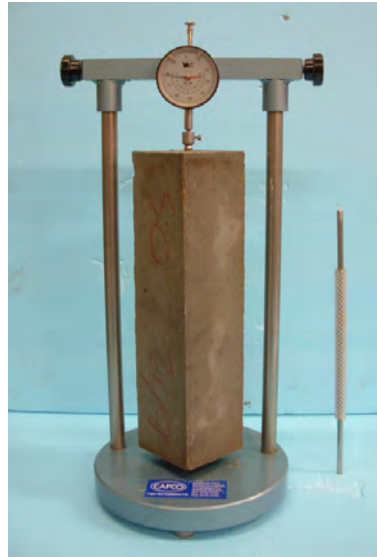
Figure 4.9: Frame used for deformation measurement.
