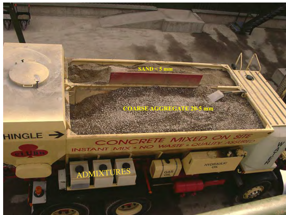
Figure 9.1: Volumetric batching plant used in the demonstration .
