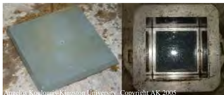
Figure 4.11: PVC insert for 150 mm special cubes [3]
