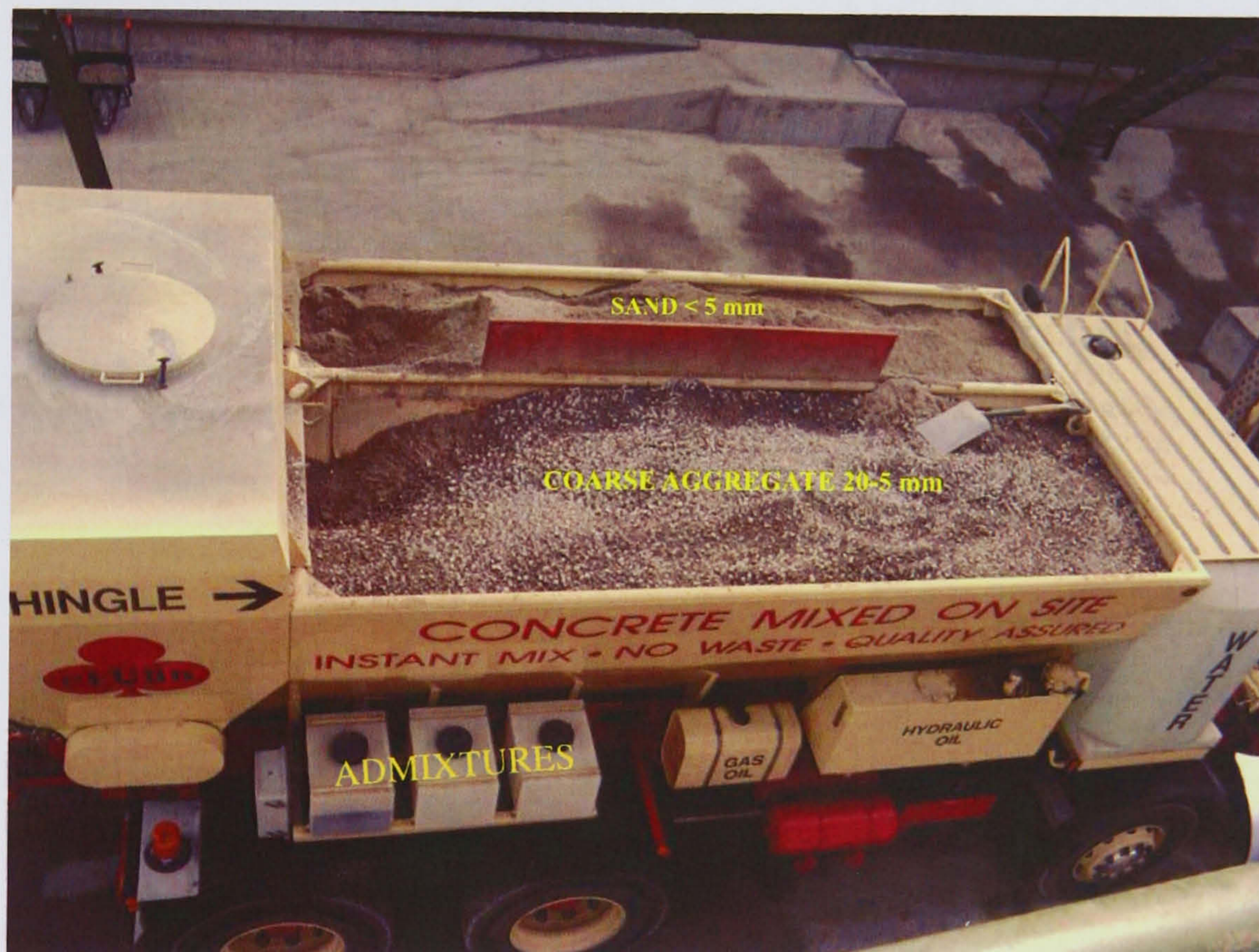
Figure 9.1: Volumetric batching plant used in the demonstration .
