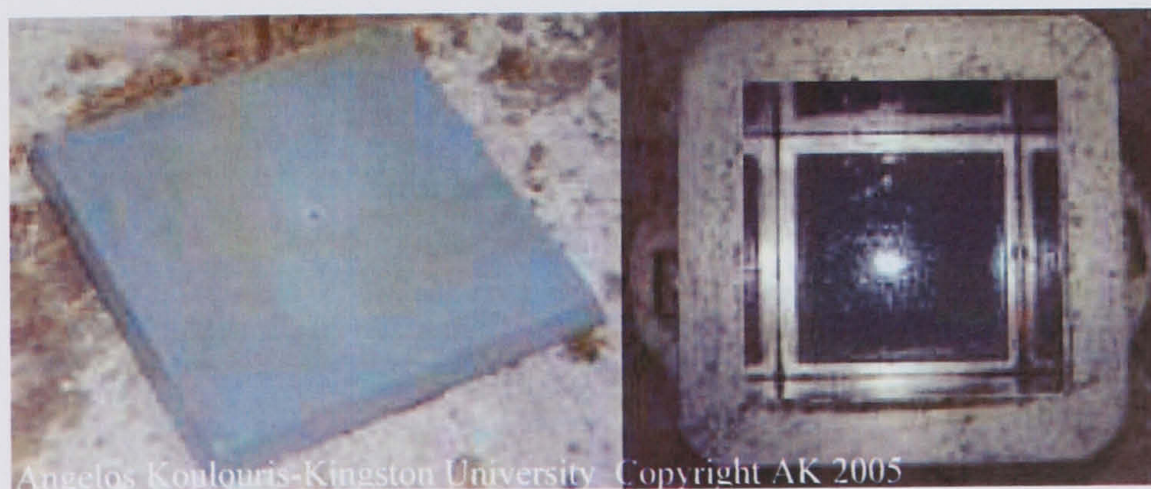
Figure 4.11: PVC insert for 150 mm special cubes [3]
