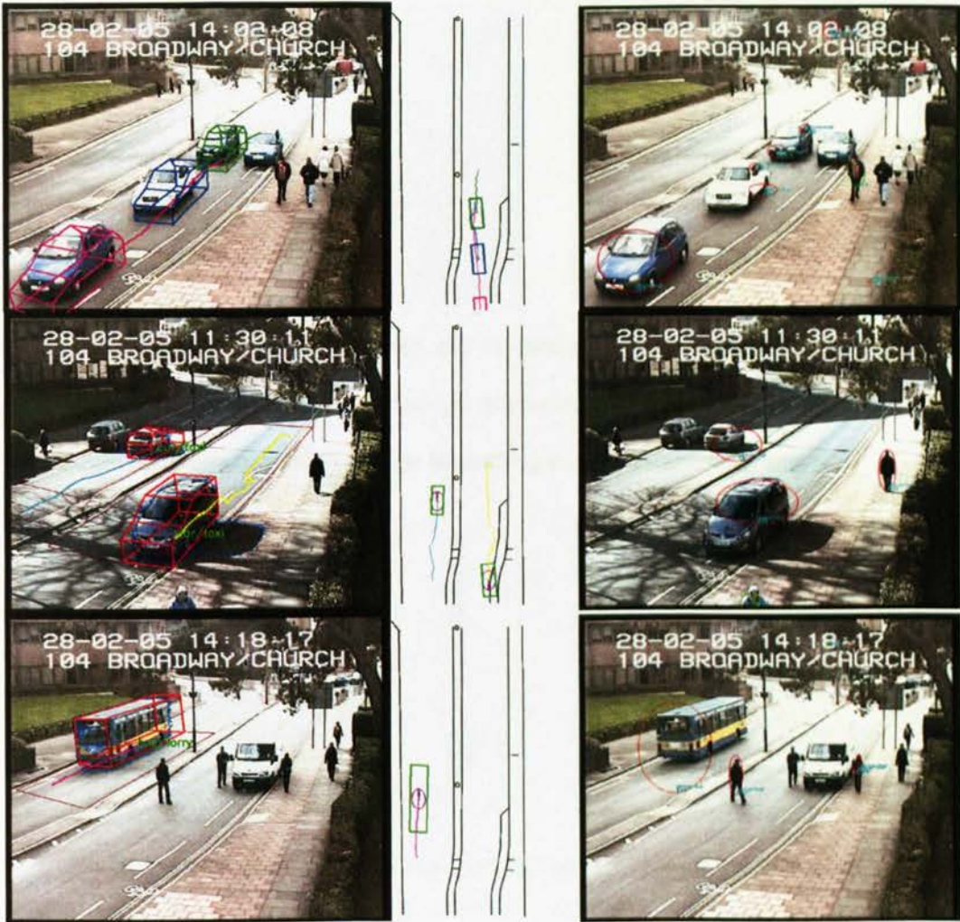
Figure 67 Correct detected tracks inside the active regions of interest (dark red boxes). Left: the proposed system with corresponding ground plane tracks. Right: OpenCV tracker result. Note the spatially fragmented tracks for the baseline in the first row and the correct number for tracks for the proposed tracker.
