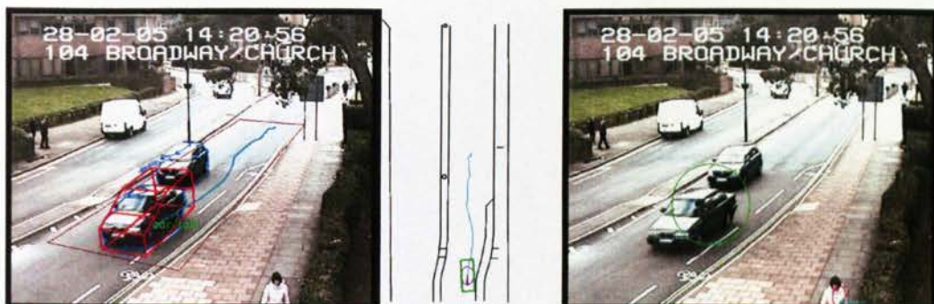
Figure 68 In this frame, the second car is missed due to occlusion between the vehicles. The proposed tracker on the left correctly locates the first car. The OpenCV tracker merged both cars with a large bounding box at a central position.
