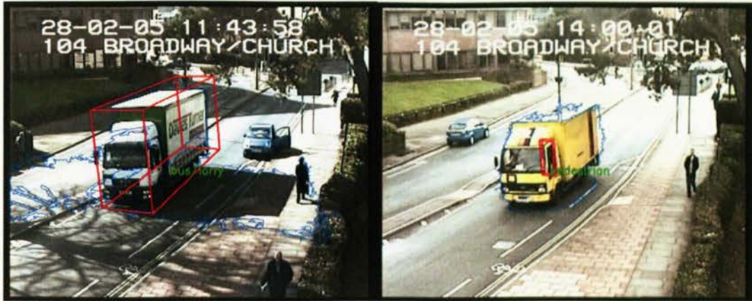
Figure 56 Left: Correctly classified lorry with 3DHOG despite shadows and oversized motion silhouette. Right: wrongly detected pedestrian at the front edge of a lorry due to vertical edges.
