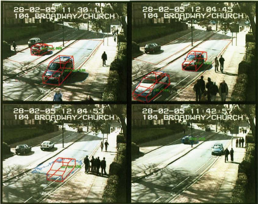
Figure 19 Sunny examples top: true positive, bottom: false positive car and missed car
