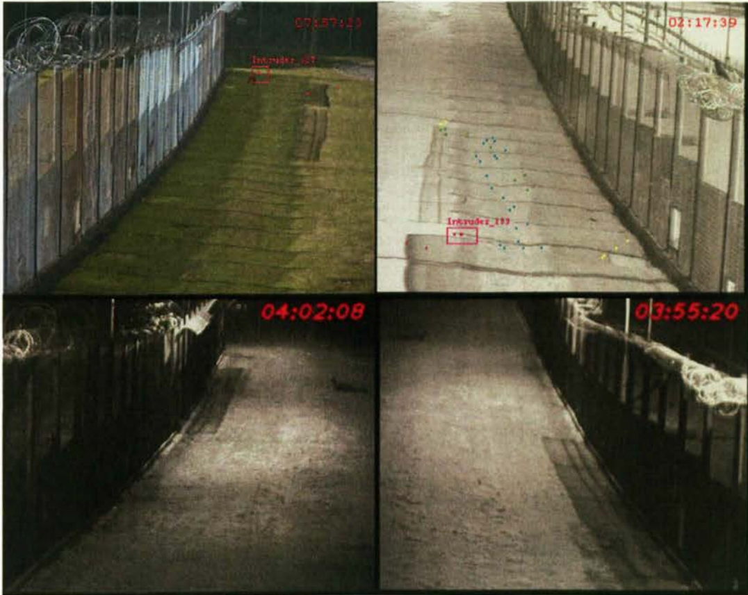
Figure 39 The top left image shows a wrongly detected bird flying towards the fence. The top right images shows a false detection due to fast moving clouds present at the same time as fence shadows, both errors are caused by texture. The bottom images show missed intruders due to low lighting conditions at night.
