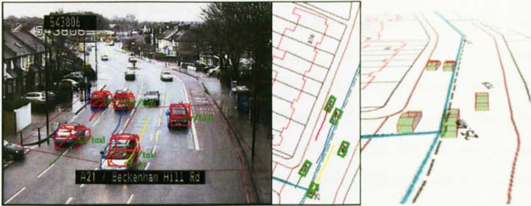
Figure 66 Example of detection and classification with ground plane tracking. The wire frame projection in red is used to estimate the bounding box for tracked vehicles. The information can be used for an anonymised animation to overcome privacy limitations of video data.
