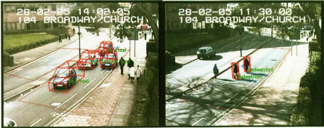
Figure 41 Example views from the i-LIDS data set with detected and classified pedestrians and vehicles using 3DHOG
