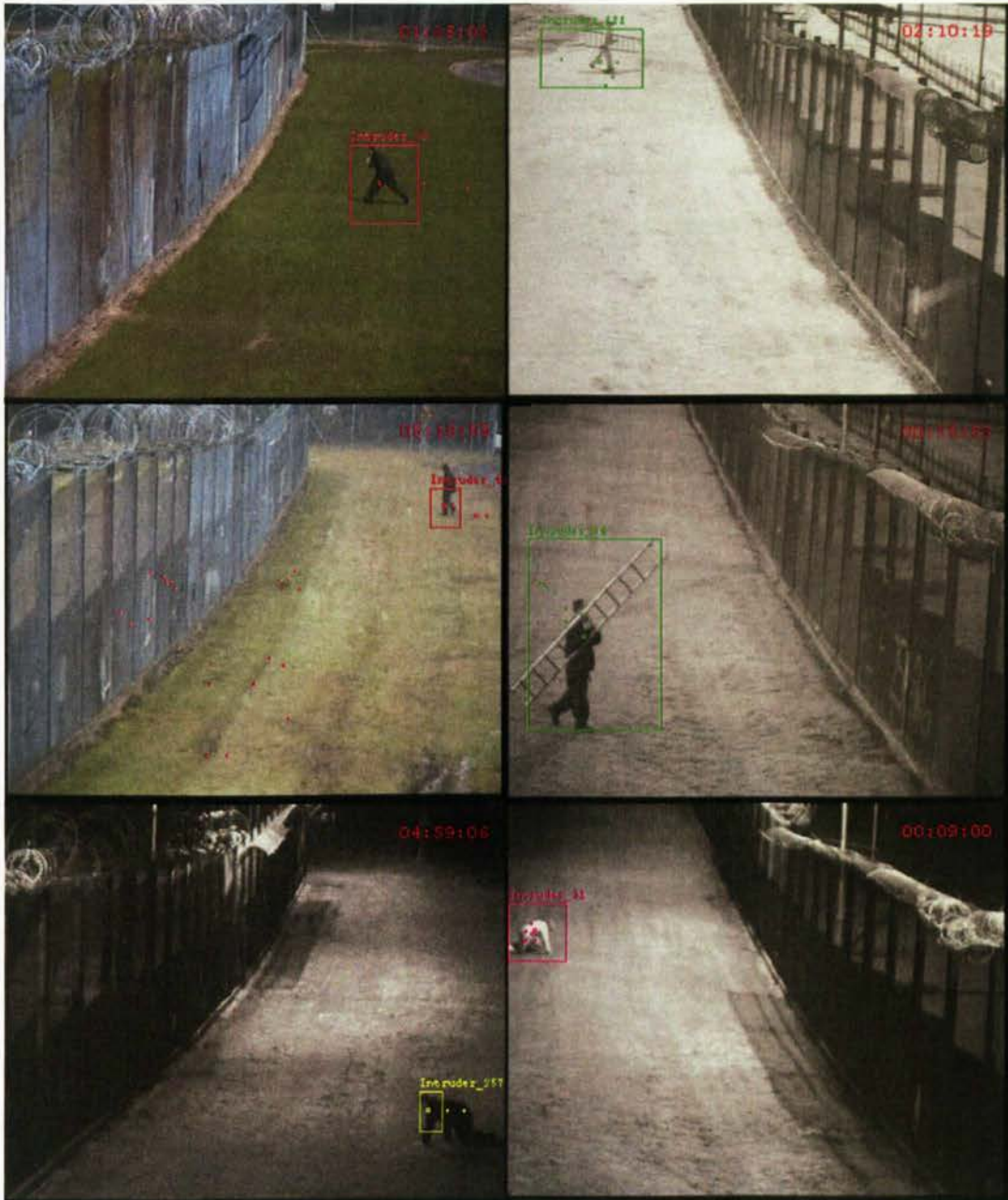
Figure 22 Examples of the i-LIDS data set showing the two camera views, different environmental conditions (falling snow in the middle left) and ways the fence is approached.
