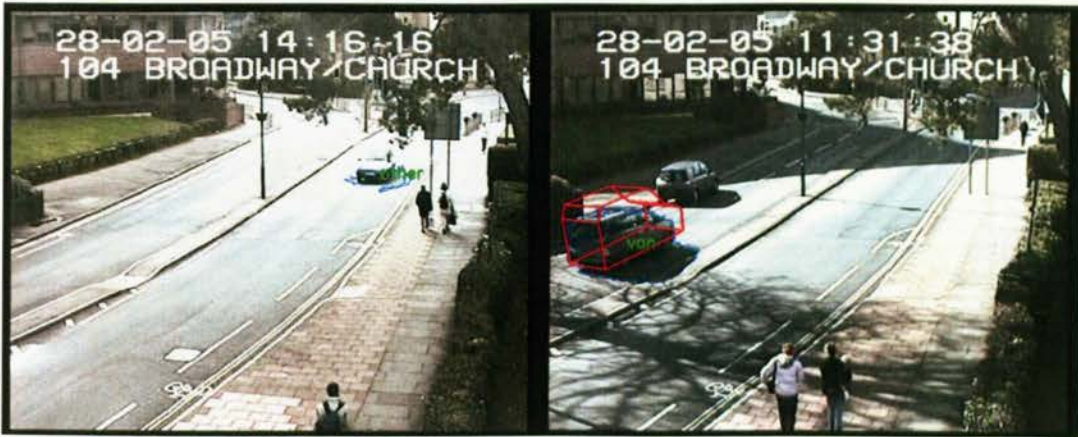
Figure 55 Two examples of errors generated with 3DHOG. Left: Missed car due to low contrast of the vehicle bonnet and roof. Right: Misclassified SUV as van due to similar size and appearance.
