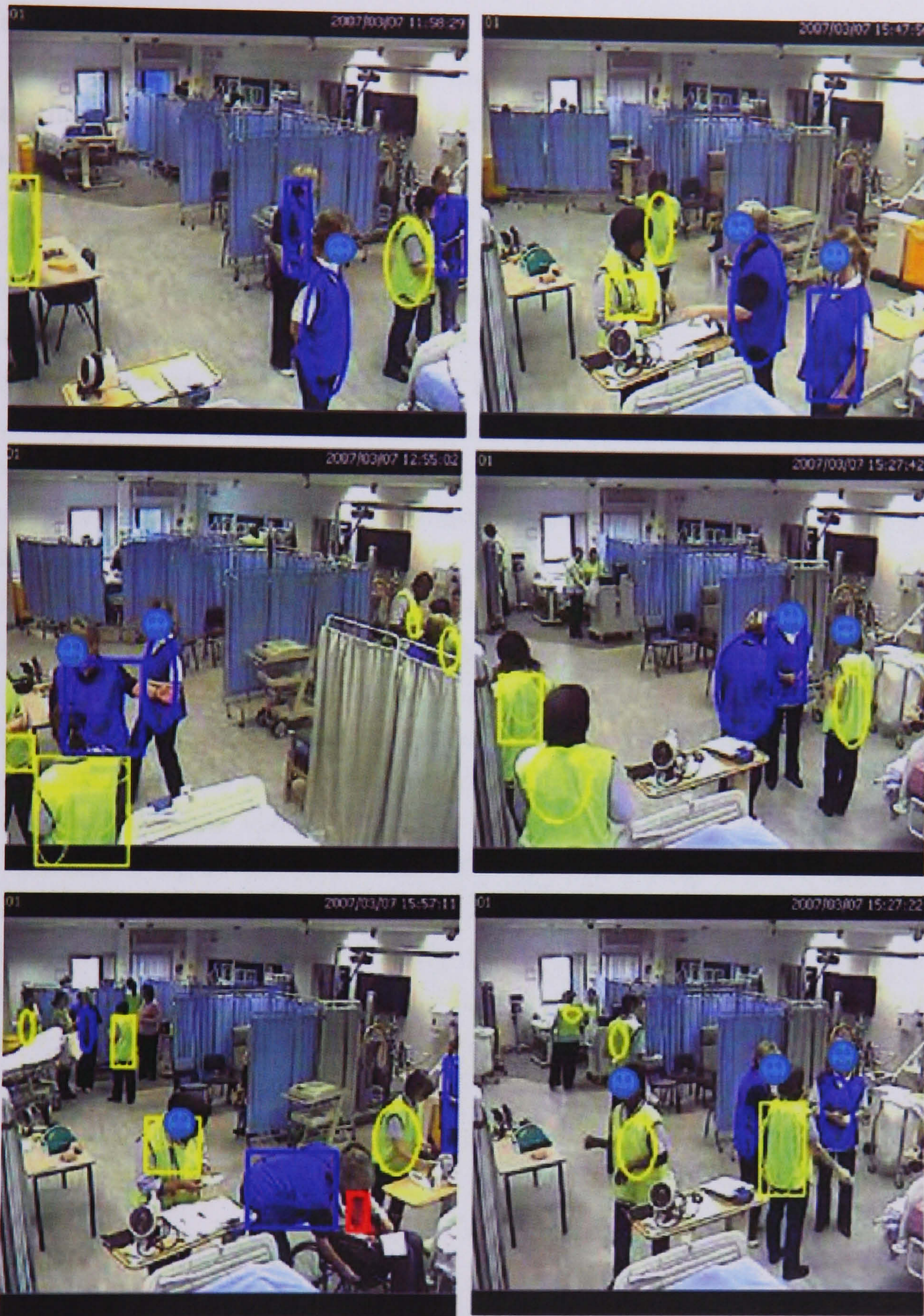
Figure 3.20: Counting people: ellipses represent the original blobs. Thick outlines of shapes show the existences of individuals. If a single colour blob is counted as an individual, the blob is displayed as an ellipse with thick outline; otherwise it is displayed with thin outline. For example, in the first graph of second row, the big yellow rectangle on the left with thick outlines is to show the existence of a nurse while the ellipses with thin outlines inside it are to show the original detected colour blobs.
