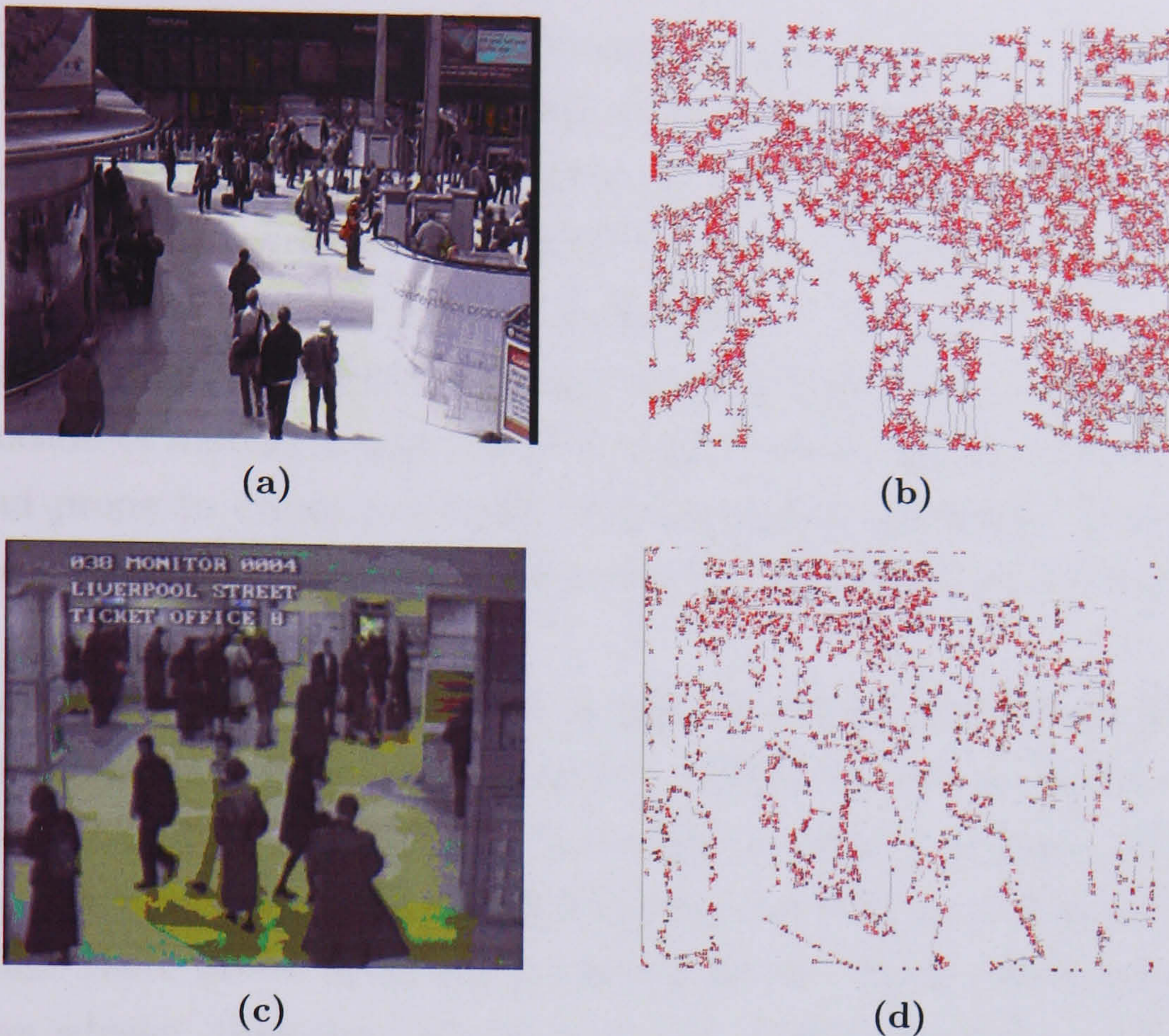
Figure 4.5: Two scenes of different complexity levels are illustrated. The original frames (left) and the extracted corner points (right) that are marked with red crosses on grey edges.
