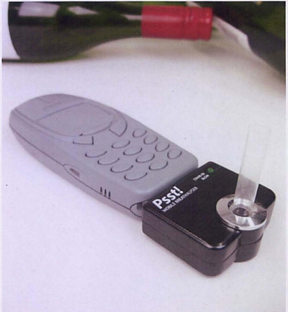
Figure 75: PSST! - alcohol breathalyser add-on unit [photo: author]
