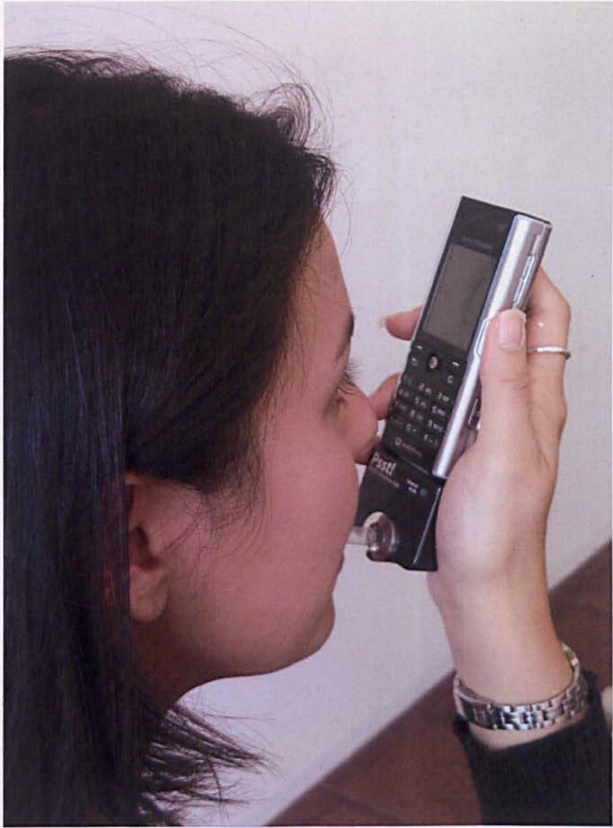
Figure 76: PSST! - Mobile phone - alcohol breathalyser in use [photo: author]
