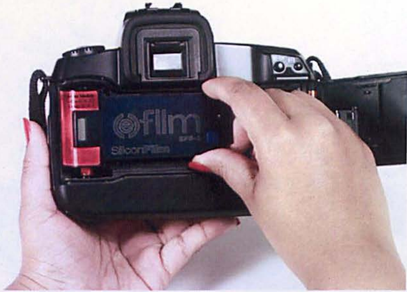
Figure 23: Piggybacking digital 'E-film' into a 35mm film camera (Siliconfilm 2005)
