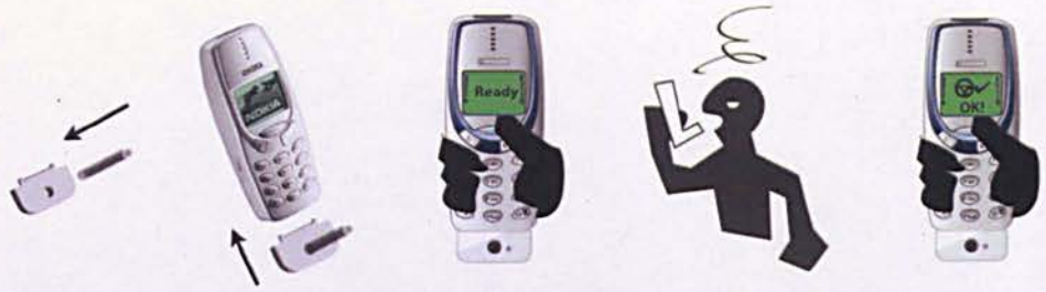
Figure 46: William – add-on module to convert a mobile phone into a breathalyser
