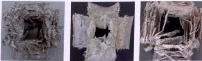
Plan view of crushed CFRP and GFRP composite box struts
