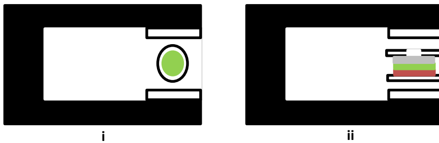
Figure 3.6 – i) The parallel set up of the device and magnetic (Para Mag) and ii) the perpendicular set up of the device and magnetic (Perp Mag)
