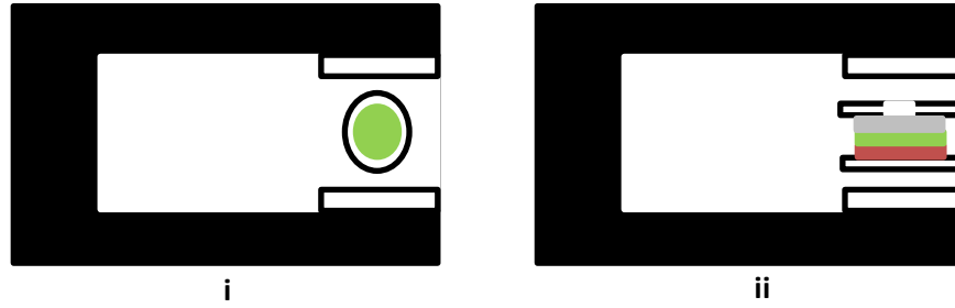
Figure 3.6 – i) The parallel set up of the device and magnetic (Para Mag) and ii) the perpendicular set up of the device and magnetic (Perp Mag)
