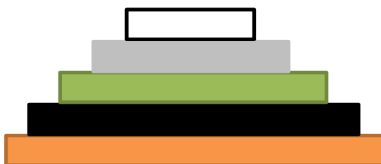
Figure 3.4 – A typical photosensitive device architecture showing the copper electrode (orange), silicon/ \text{FePS}_3 substrate (black), nanocomposite material (green) ITO coated on PET (grey) and the plastic plate (white)
