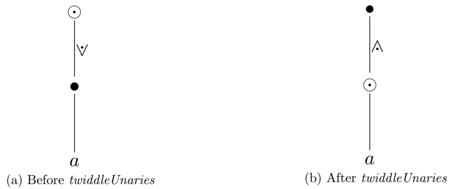
Figure A.7: twiddleUnaries tree transformation for representation of \odot a \bullet where \bullet is a postfix operator, \odot is prefix (or \bullet is prefix and \odot postfix), and \odot \succ \bullet
