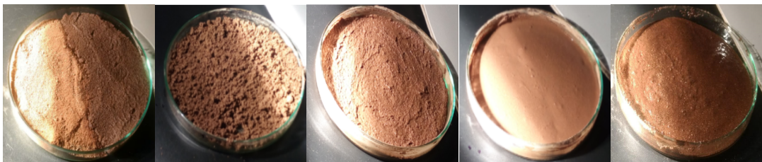
FIGURE 4.5: Sample preparation of the experiment combining sandy - loam with diesel. Photos show the HC contaminant being increasingly added to the same soil sample until saturated. From left; addition of 5ml , followed by 10ml, 15ml, 20ml and 25ml of the HC
