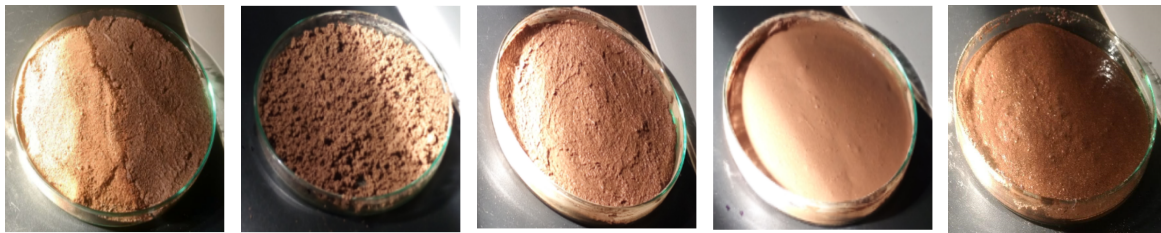
Figure 1. Sample preparation of the experiment combining sandy-clay-loam with diesel. Photos show the HC contaminant being increasingly added to the same soil sample until saturated. From left; addition of 5 mL, followed by 10 mL, 15 mL, 20 mL, and 25 mL of the HC.
