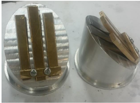
Figure 4-36: Reed Valves Angled at 40°
