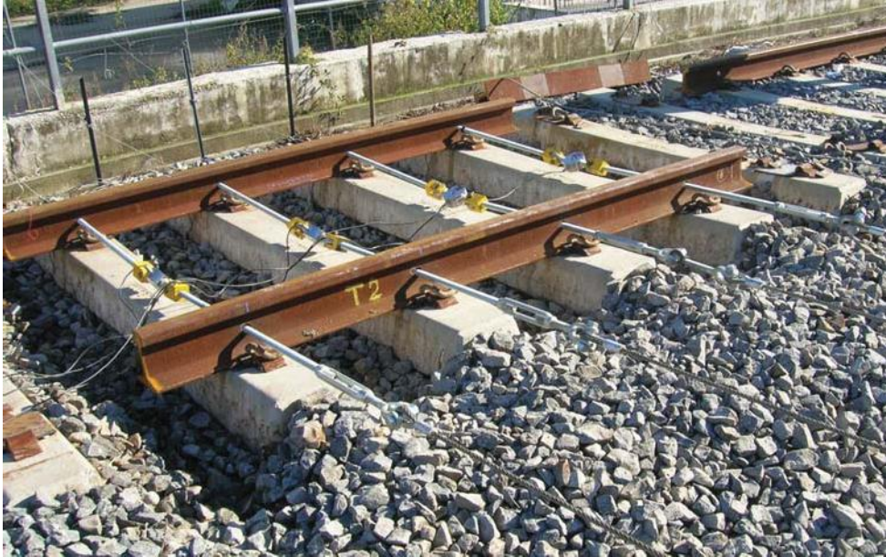
Figure 6. Test on BCB scenario (without ballast crib - C).
