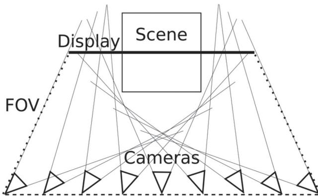
**FIGURE 3** Arrangement of the linear camera array
