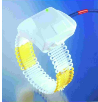
Figure 2.2: The transducer band used in Filtrass (Filtrass, Munich, Germany) [own photo]
