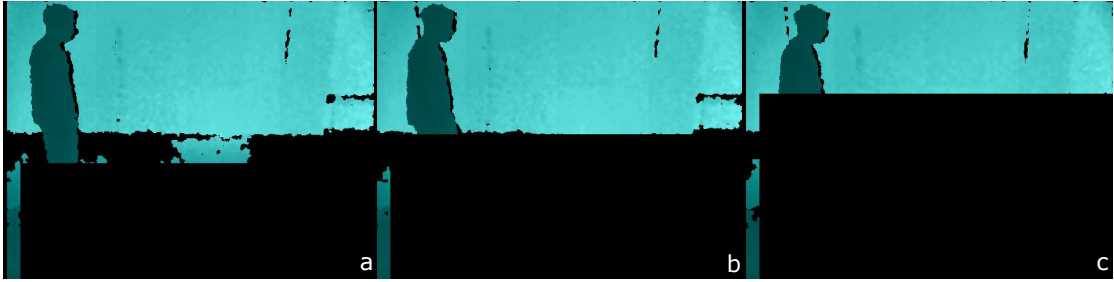
FIGURE 7.1: Three occlusion modes. The black rectangle in the image is a synthetic occlusion applied to the depth image. The degree of occlusion is expressed proportionally to the person's height: (a) 40%, (b) 50%, (c) 70% occlusion measured from the ground
