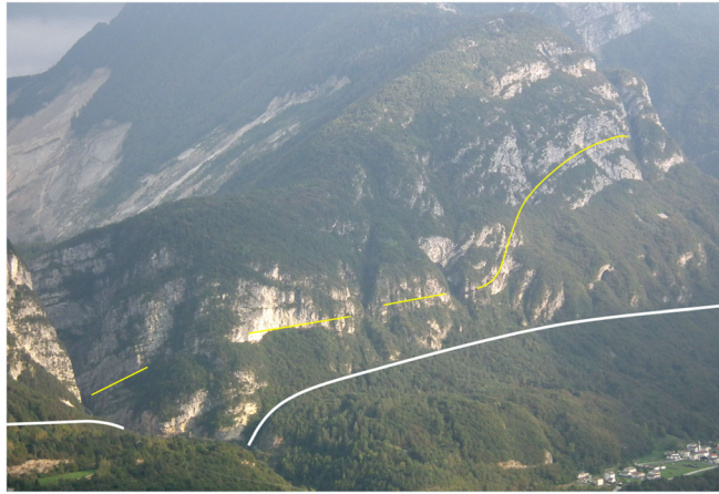
Fig. 7 Left wall of the Piave Valley above Longarone in September 2011, showing the ‘chair’ structure (bedding indicated by yellow lines) that was mistakenly assumed to extend beneath at least the western half of the landslide. The white line marks the alignment of the Col delle Tosatte Fault. The downstream end of the Vaiont Gorge is at the lower left of the image and part of the landslide scar is visible in the upper left part. Photo: APD
