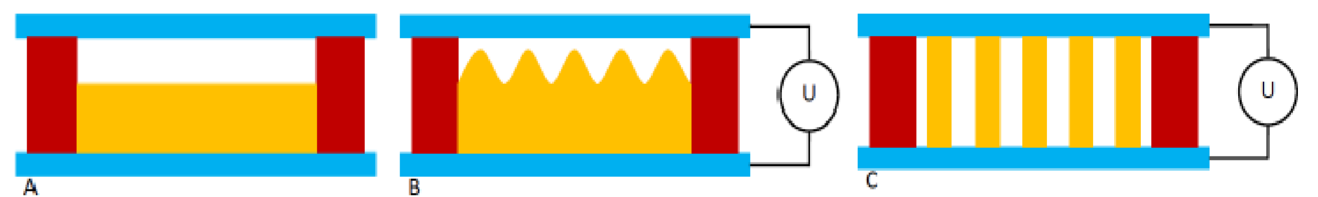
Fig. 3 blue-electrode, red-spacer, yellow-fluid A. no applied voltage B. initial instability C. fully evolved structures
