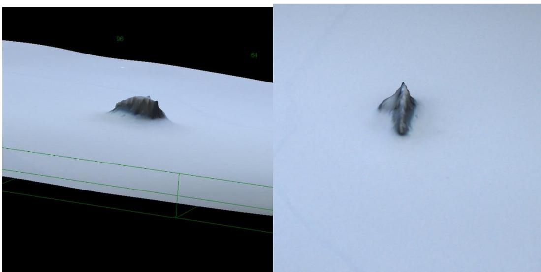
Figure 5. Example showing two views of the same sharp volcanic fragment (6 by 12  $\mu\text{m}$ ) from sample C Grimsvötn eruption.
