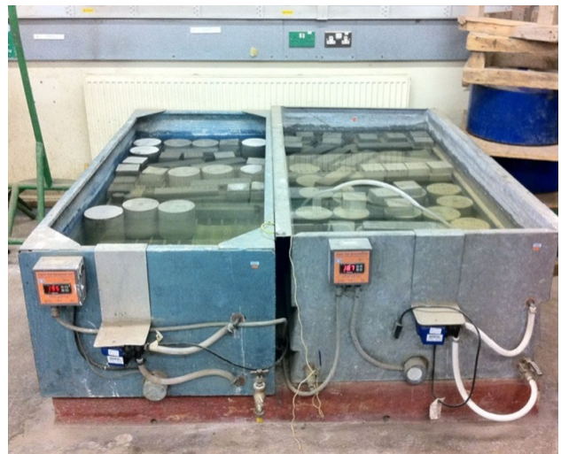
Figure 5. Concrete cubes under water curing environment (C3).
