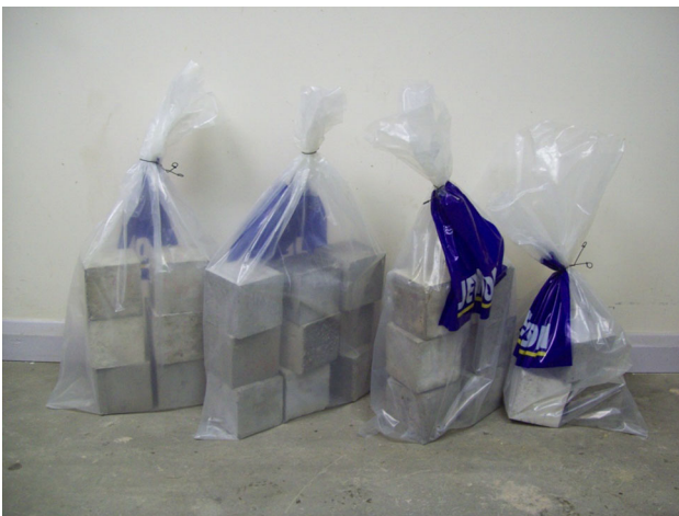
Figure 3. Test cubes under summer curing environment (C1).
