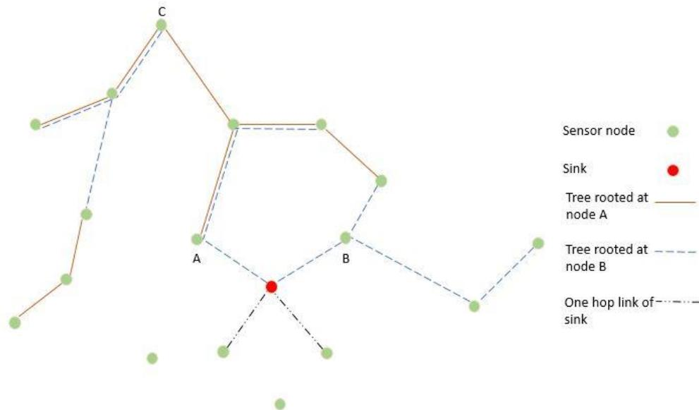
*Figure 2-1: Sequential assignment routing. (Rao, et al., 2003, Sept. )*
