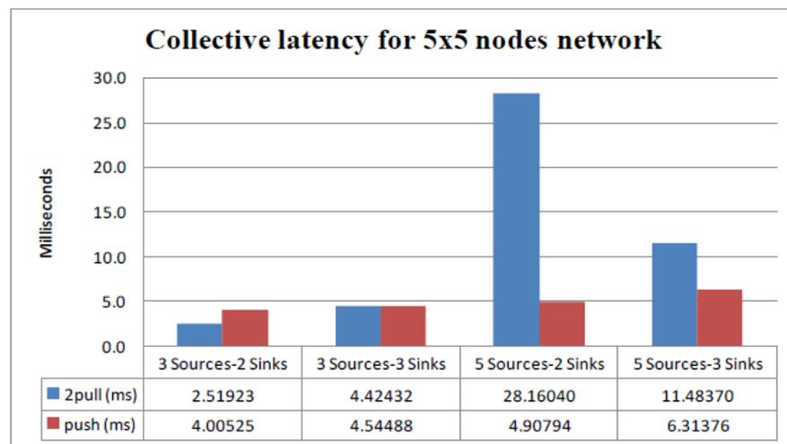
*Figure 3-7: The collective latency in 5x5 nodes network*
