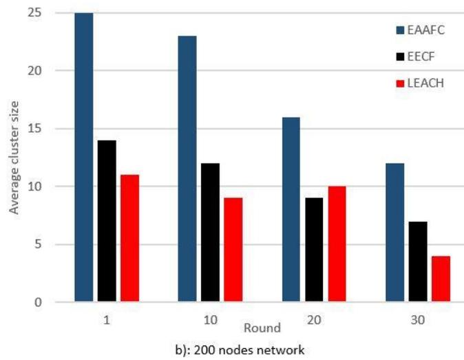
**Figure 4-5: Average cluster sizes comparison for EAAFC, EECF, LEACH and highest-Degree**
