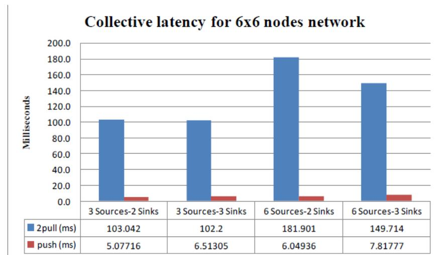
*Figure 3-8: The Collective Latency in 6X6 nodes network*
