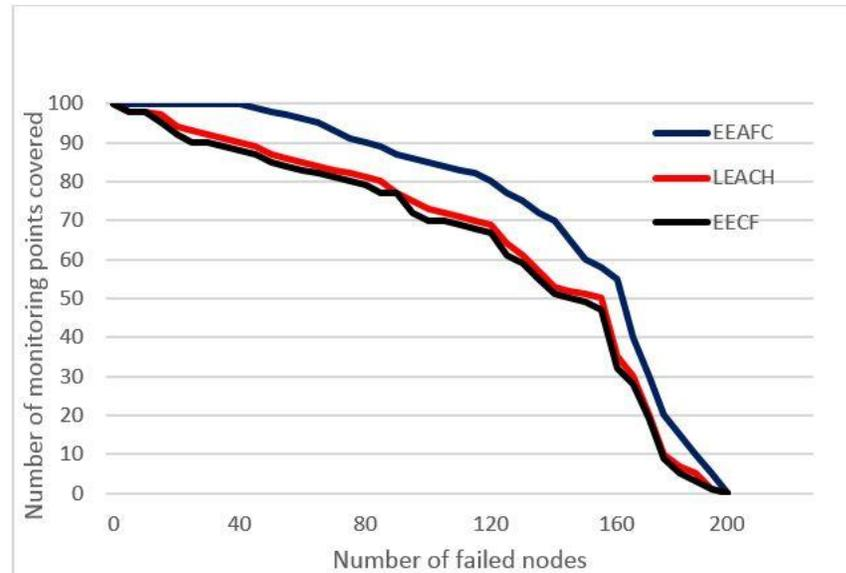
**Figure 4-10 Network coverage with several dead nodes**
