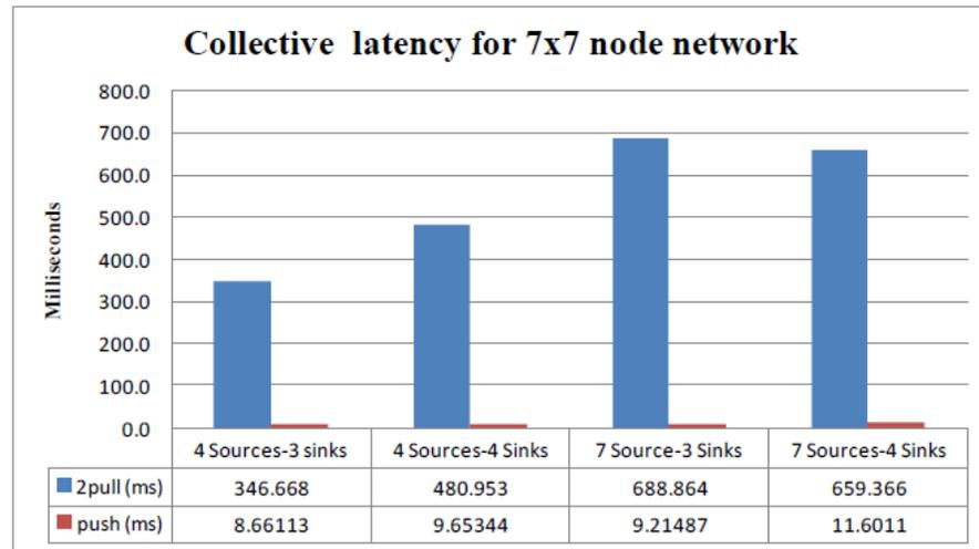
***Figure 3-9: The collective latency in 7x7 nodes network***
