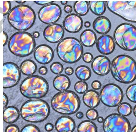
d. Fill factor 0.35; E-field in polymer  $0.68 \text{ MV m}^{-1}$ ; image width  $257 \mu\text{m}$
