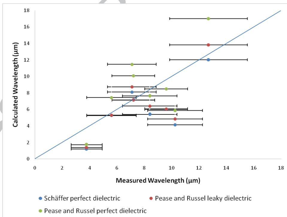
Figure 6. Graph of experimental results vs. theoretical values for wavelengths below  $15\mu\text{m}$ .
