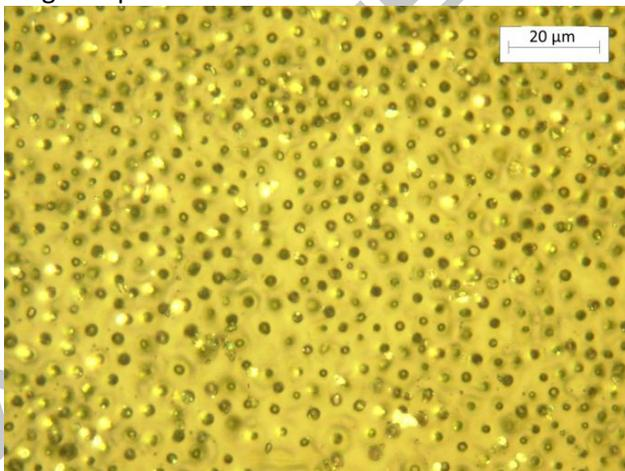
c. Epoxy fill factor 0.77; field  $22.7 \text{ MV m}^{-1}$ ; pattern height  $3 \mu\text{m}$ . Lighter areas are where the epoxy disks have adhered to the top electrode and detached from the surface.
