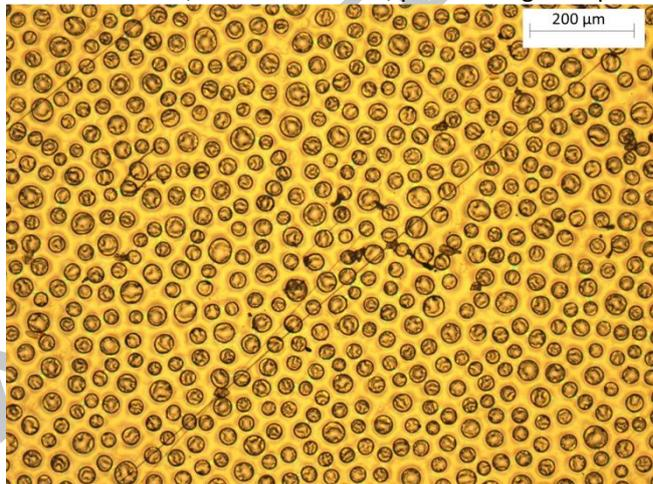
e. Fill factor 0.28; field  $1.01 \text{ MV m}^{-1}$ ; pattern height  $8.9 \mu\text{m}$
