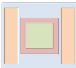
Figure 2. Bottom electrode configuration. Blue: glass slide; pink: etched ITO; orange: spacer; green: epoxy layer on top of ITO.
