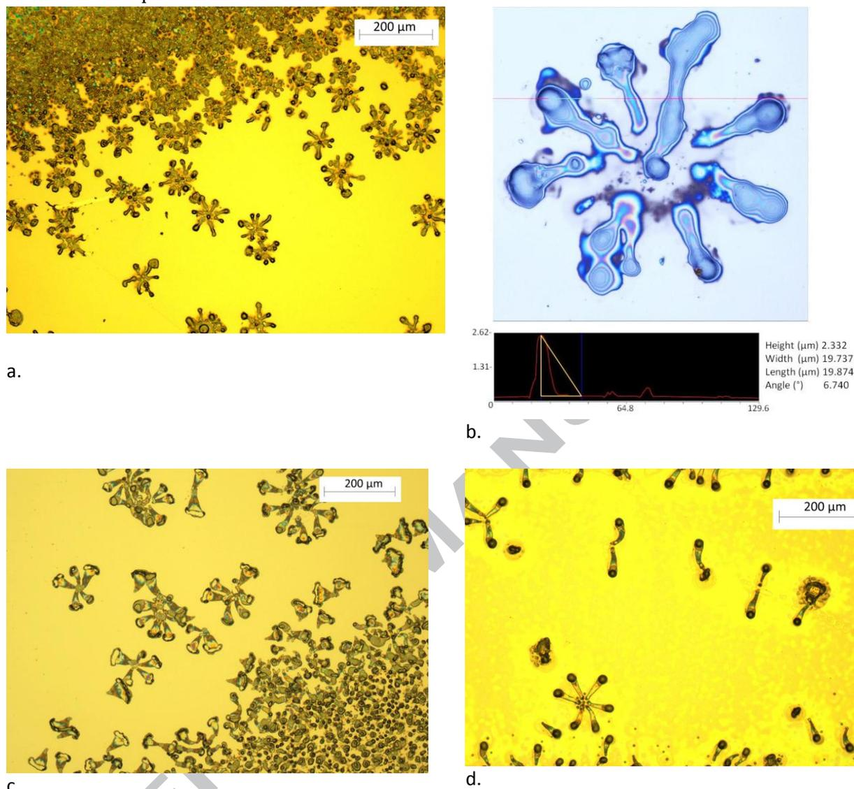
Figure 11. a: Starburst effect. Epoxy thickness  $0.5\ \mu\text{m}$ ; spacer  $2.3\ \mu\text{m}$ . b: 3D LEXT examination of the epoxy patterns left on the two electrodes, showing that the material had fanned out whilst being in contact with both electrodes. c: Starburst effect. d: Starburst and traversing pillars.
