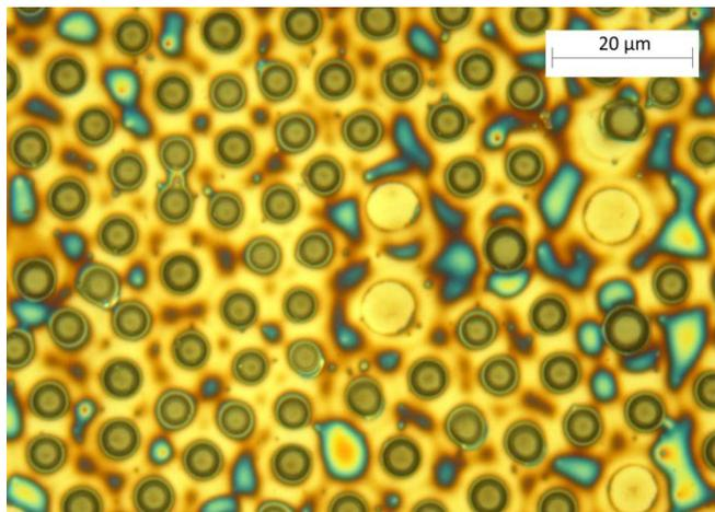
a. Fill factor 0.5; field  $6.5 \text{ MV m}^{-1}$ ; pattern height  $2 \mu\text{m}$
