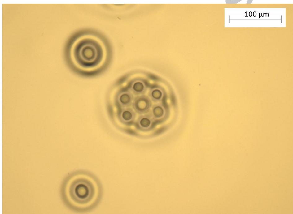
Figure 3. Optical micrograph showing a quasi-hexagonal patterned array forming around a central pillar. Pattern height: 26.6 $\mu\text{m}$
