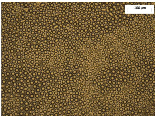
c. Fill factor 0.27; field  $1.28 \text{ MV m}^{-1}$ ; pattern height  $9.6 \mu\text{m}$
