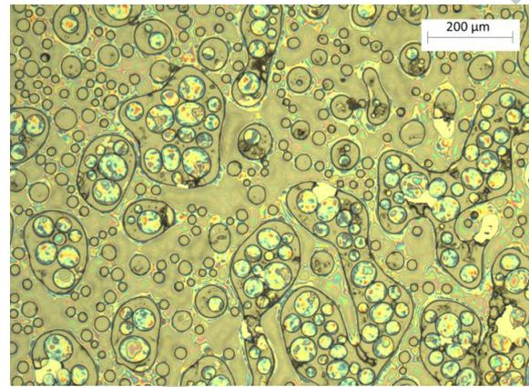
b. Fill factor 0.58; E-field in polymer  $0.94 \text{ MV m}^{-1}$
