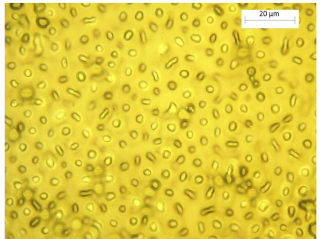
d. Epoxy fill factor 0.6; field  $8.39 \text{ MV m}^{-1}$ ; pattern height  $3.1 \mu\text{m}$ .
