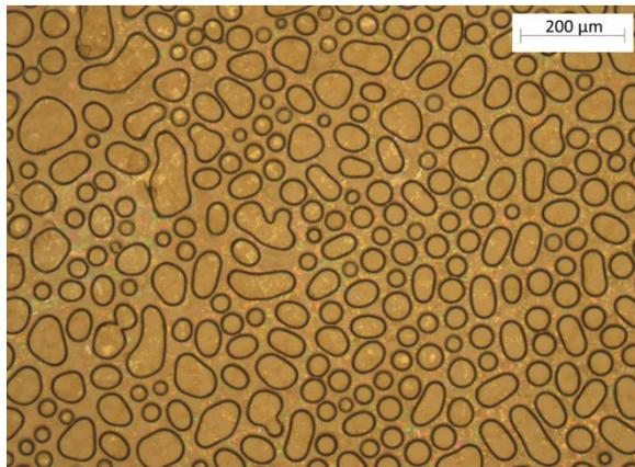
a. Fill factor 0.45; E-field in polymer  $2.2 \text{ MV m}^{-1}$
