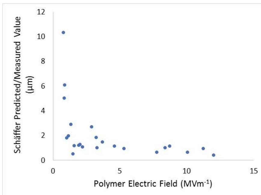
Figure 7. Plot of the ratio of predicted to measured wavelengths vs. the polymer electric field. (A perfect dielectric sample with a relative permittivity of 9.0 was assumed.)
