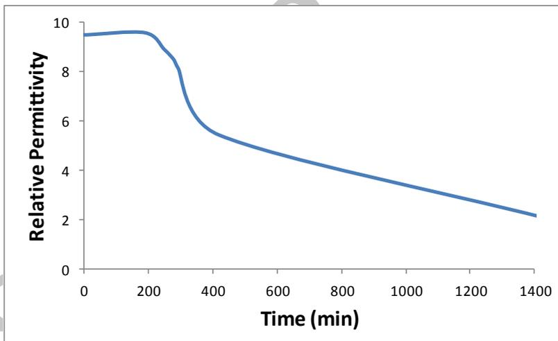
Figure 8. Graph showing the change in the relative permittivity of the epoxy resin as a function of curing time.
