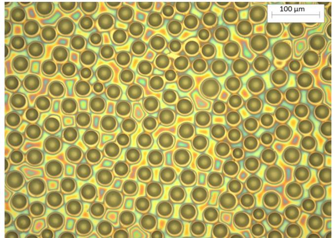
f. Fill factor 0.32; field  $2.48 \text{ MV m}^{-1}$ ; pattern height  $4.9 \mu\text{m}$
