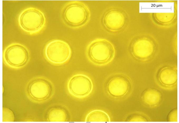
b. Fill factor 0.26; field  $0.883 \text{ MV m}^{-1}$ ; pattern height  $26.6 \mu\text{m}$
