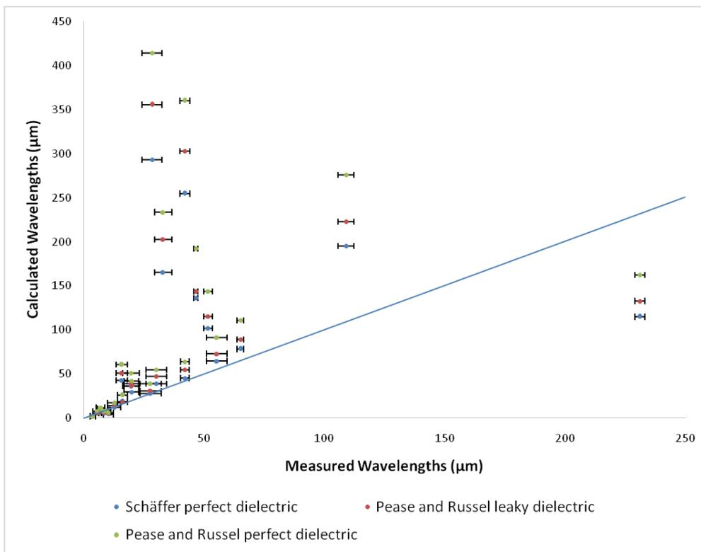
Figure 5. Graph of measured experimental results vs theoretically predicted values for the corresponding experimental parameters, taking  $\epsilon_p$  to be 9.0.
