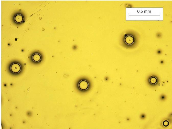
a. Epoxy fill factor 0.53; field  $2.35 \text{ MV m}^{-1}$ ; pattern height  $17 \mu\text{m}$
