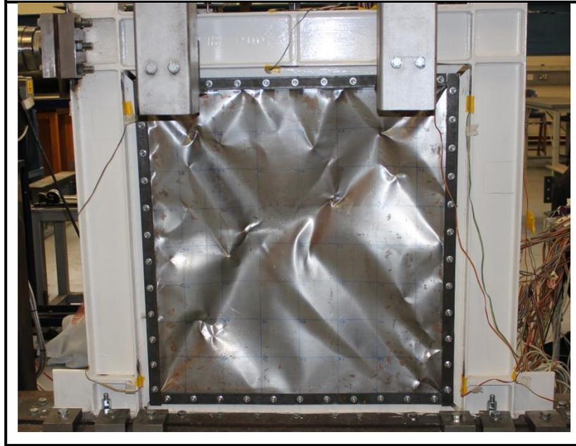
Figure 5.2. SSW\* specimen at 25 mm displacement.
