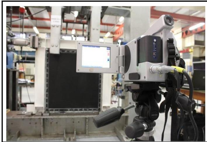
Figure 5.15. IRT camera set-up during testing.
