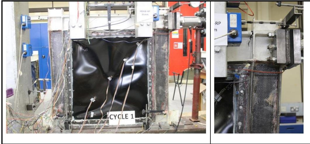
Figure 7.10. HGSW-R specimen tested to 35 mm.
